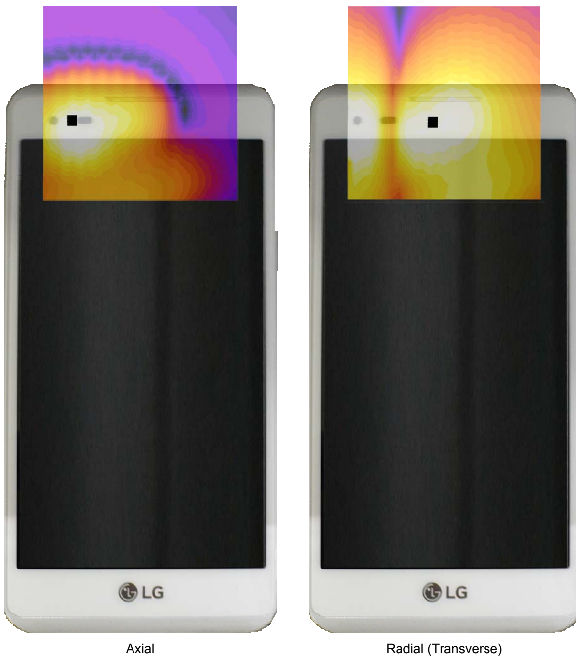
Figure 13-3 T-Coil Scan Overlay Magnetic Field Distributions
