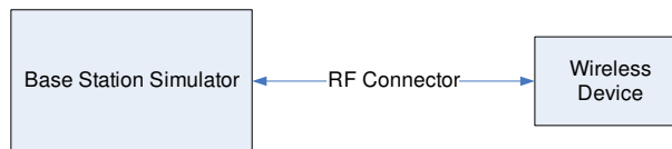
Figure 9-4 Power Measurement Setup
