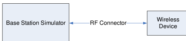
Figure 9-2 Power Measurement Setup
