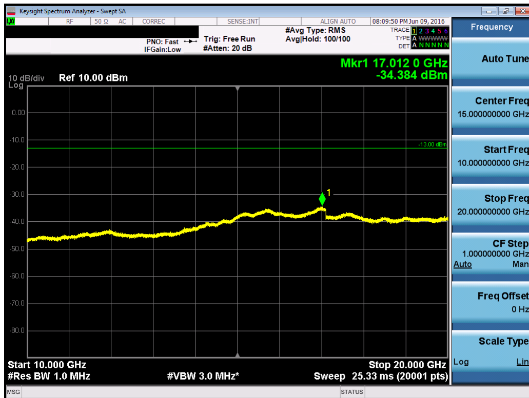
Plot 7-39. Conducted Spurious Plot (PCS CDMA Mode – Ch. 25)
