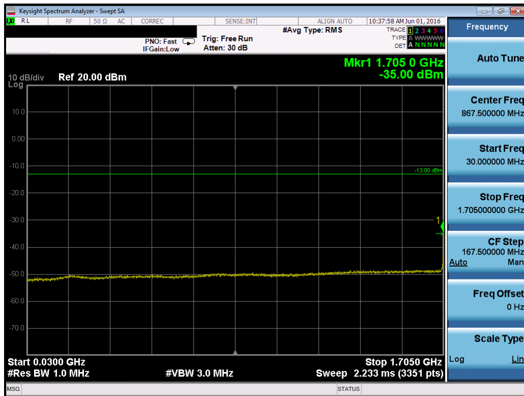
Plot 7-55. Conducted Spurious Plot (AWS WCDMA Mode – Ch. 1312)
