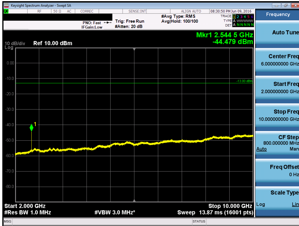
Plot 7-36. Conducted Spurious Plot (Cellular CDMA Mode – Ch. 777)
