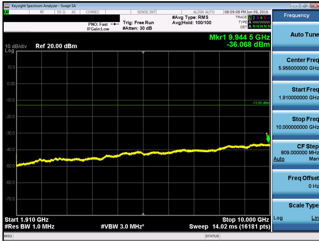
Plot 7-38. Conducted Spurious Plot (PCS CDMA Mode – Ch. 25)
