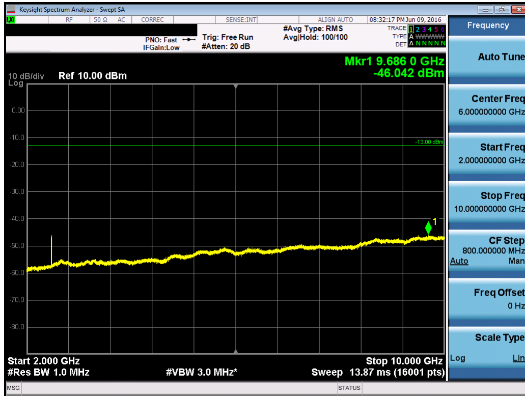
Plot 7-30. Conducted Spurious Plot (Cellular CDMA Mode – Ch. 1013)
