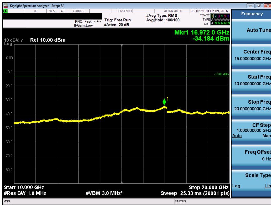
Plot 7-45. Conducted Spurious Plot (PCS CDMA Mode – Ch. 1175)
