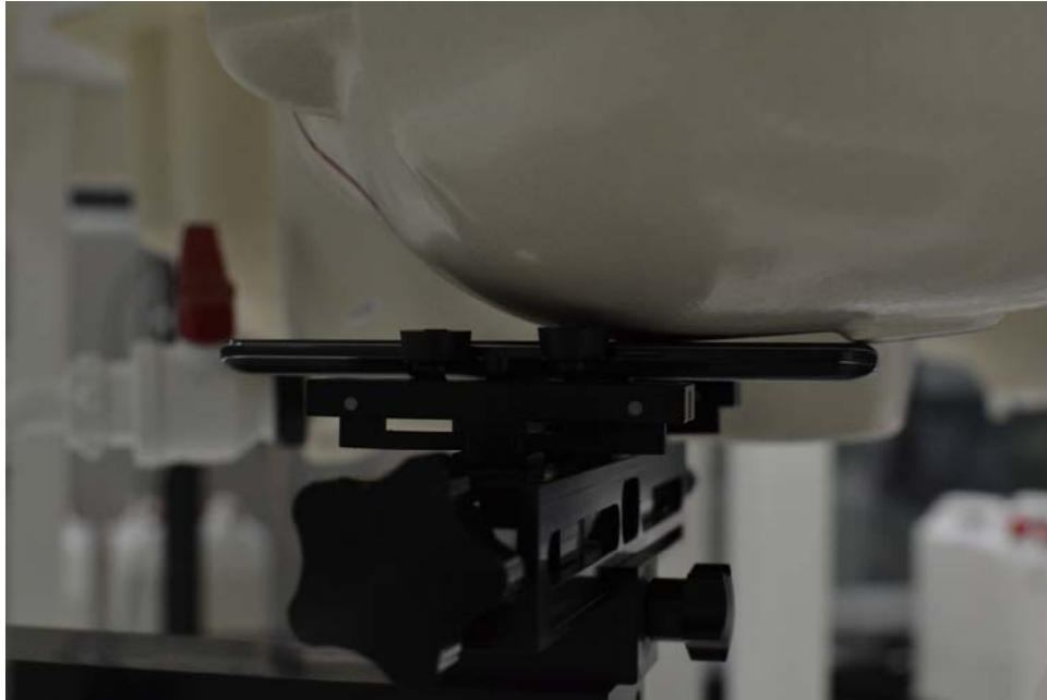
SAR Test Setup Photo 3 – Left Cheek
