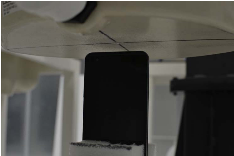
SAR Test Setup Photo 8 – Top at 10 mm
