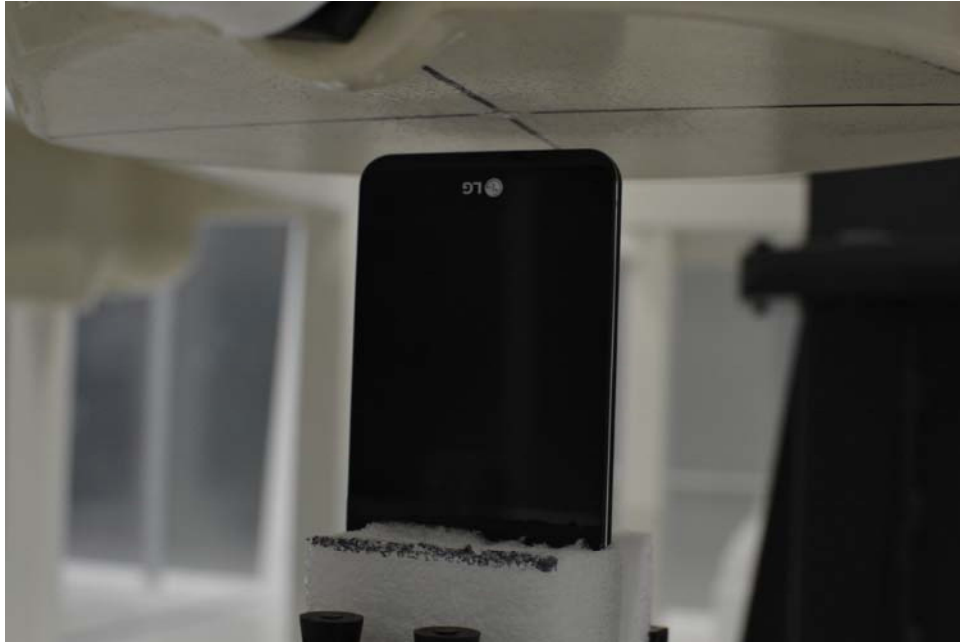
SAR Test Setup Photo 7 – Bottom at 10mm
