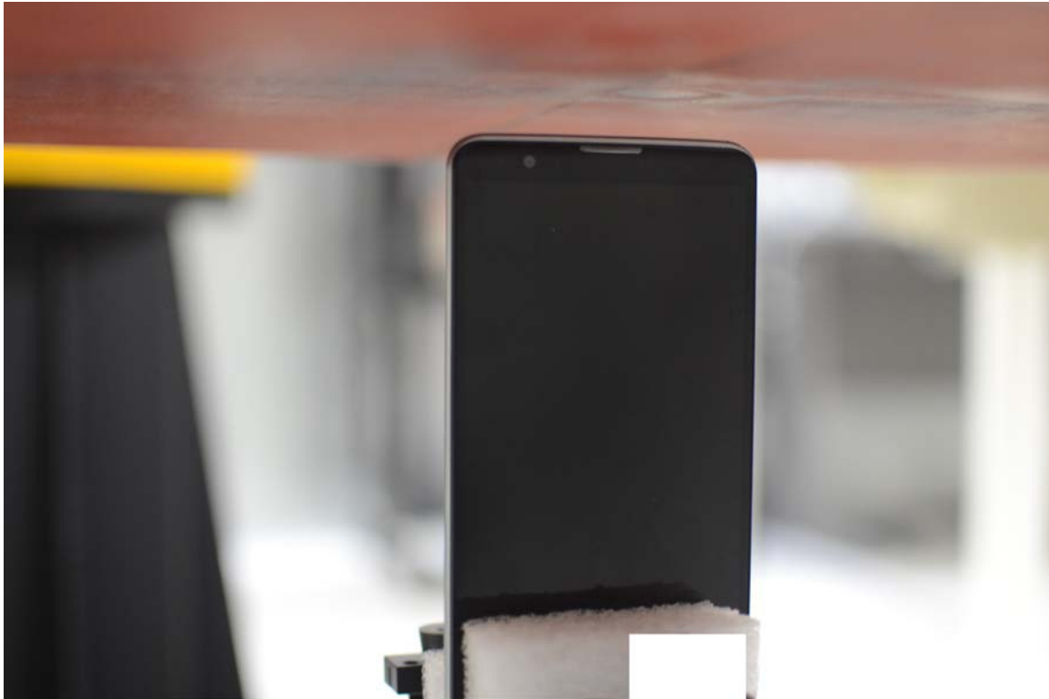
SAR Test Setup Photo 7 – Top Edge (10 mm)
