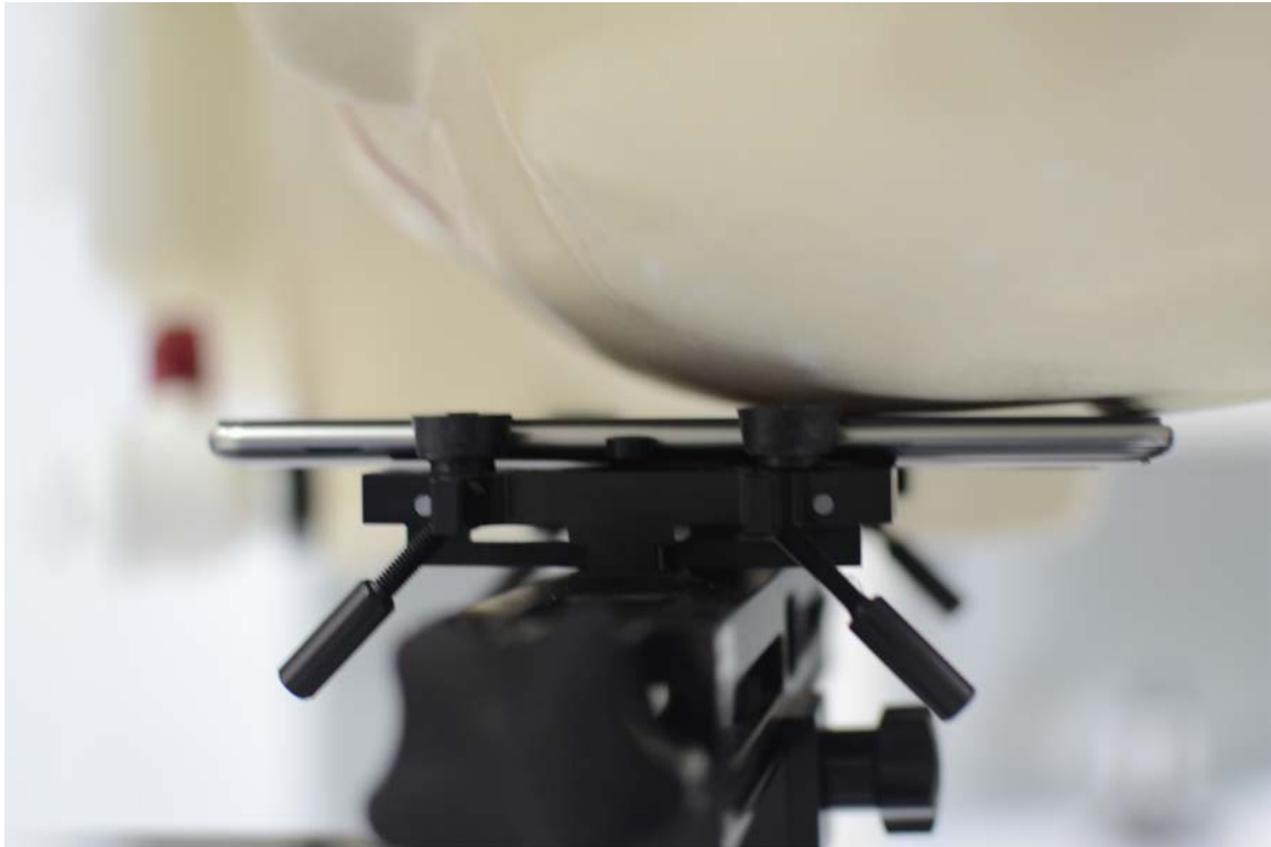
SAR Test Setup Photo 3 – Left Cheek
