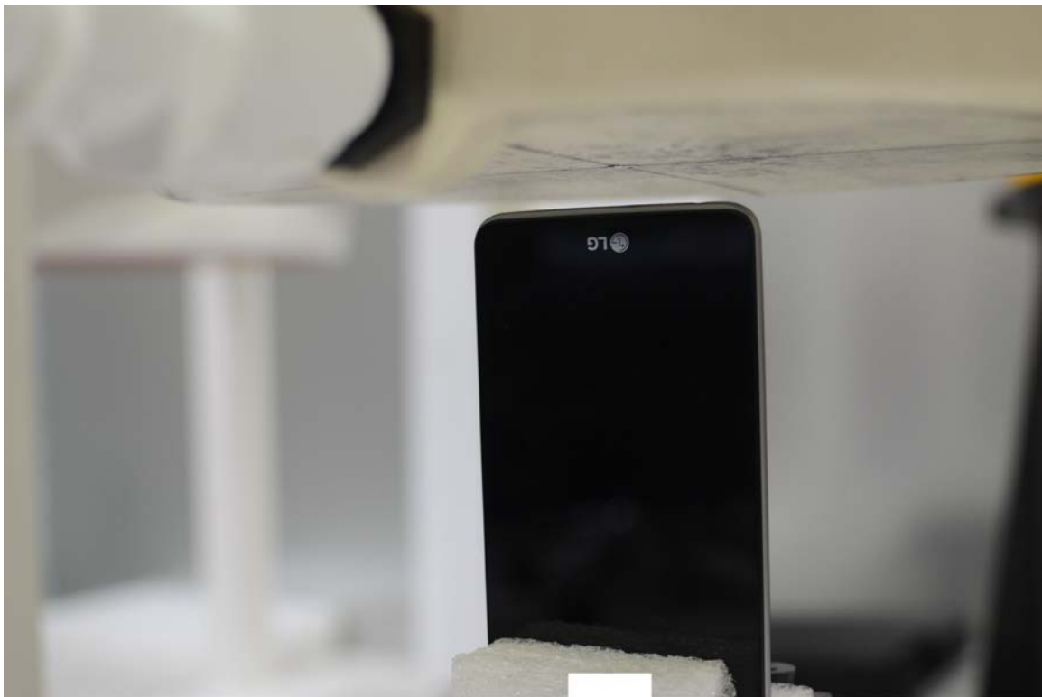
SAR Test Setup Photo 8 – Bottom Edge (10 mm)
