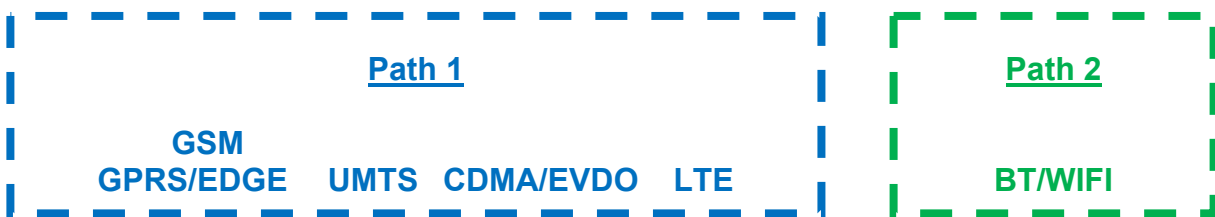
Figure 1-1 Simultaneous Transmission Paths
