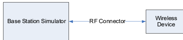
Figure 9-1 Power Measurement Setup
