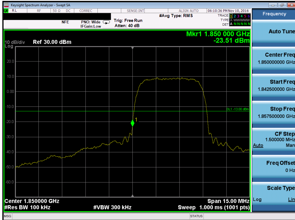
Plot 7-93. Band Edge Plot (PCS WCDMA Mode – Ch. 9262)
