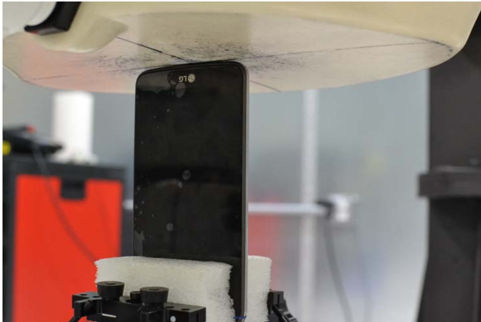
SAR Test Setup Photo 11- Bottom Edge at 0 mm
