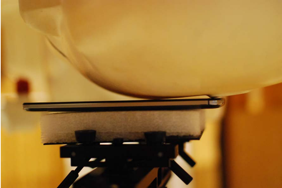
SAR Test Setup Photo 3- Left Cheek
