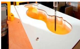
Figure 6-2 SAM Phantom with Simulating Tissue
