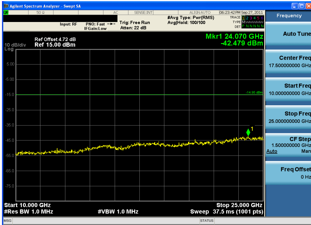
Plot 6-19. Conducted Spurious Plot (Bluetooth, 3Mbps – Ch. 39)
