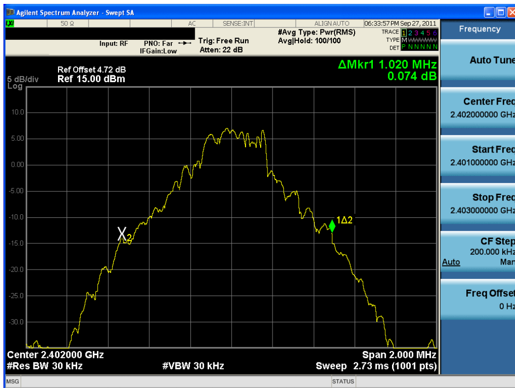
Plot 6-1. 20dB Bandwidth Plot (Bluetooth, 1Mbps – Ch. 0)
