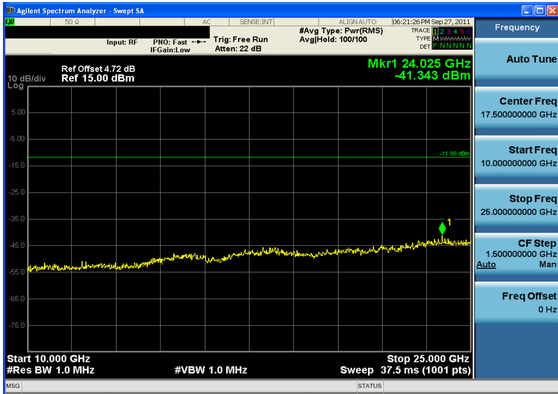
Plot 6-17. Conducted Spurious Plot (Bluetooth, 3Mbps – Ch. 0)
