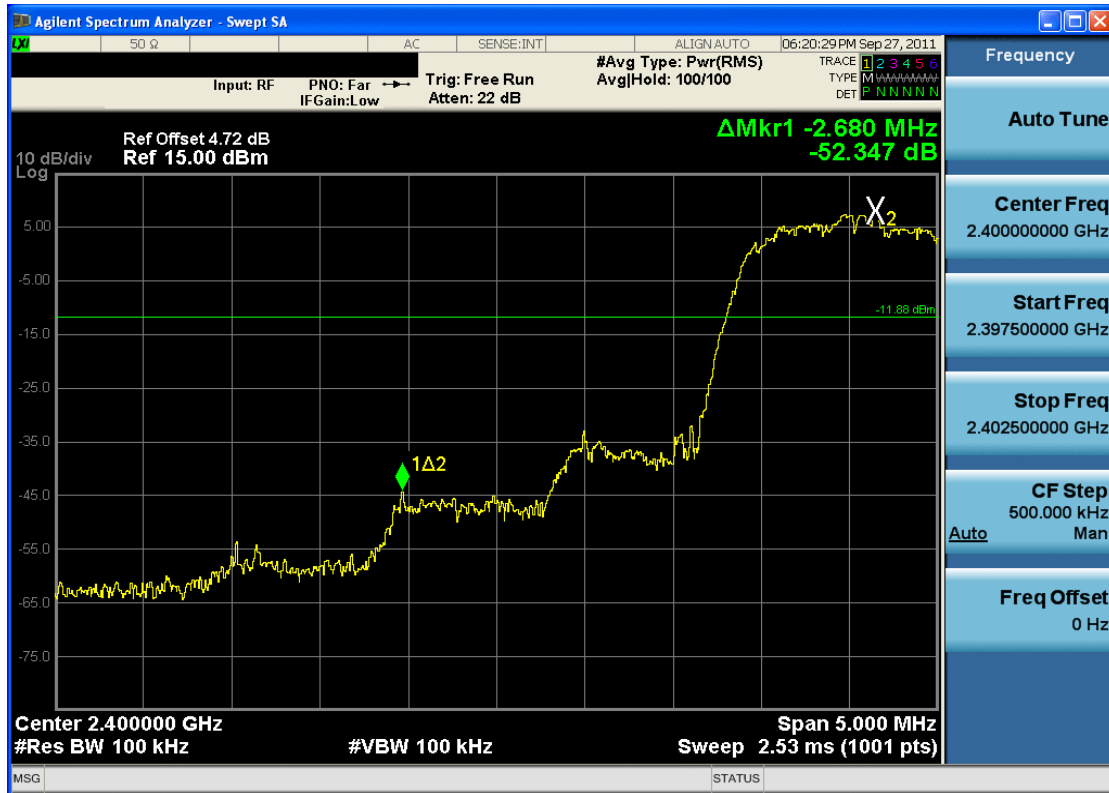
Plot 6-10. Band Edge Plot (Bluetooth, 3Mbps – Ch. 0)
