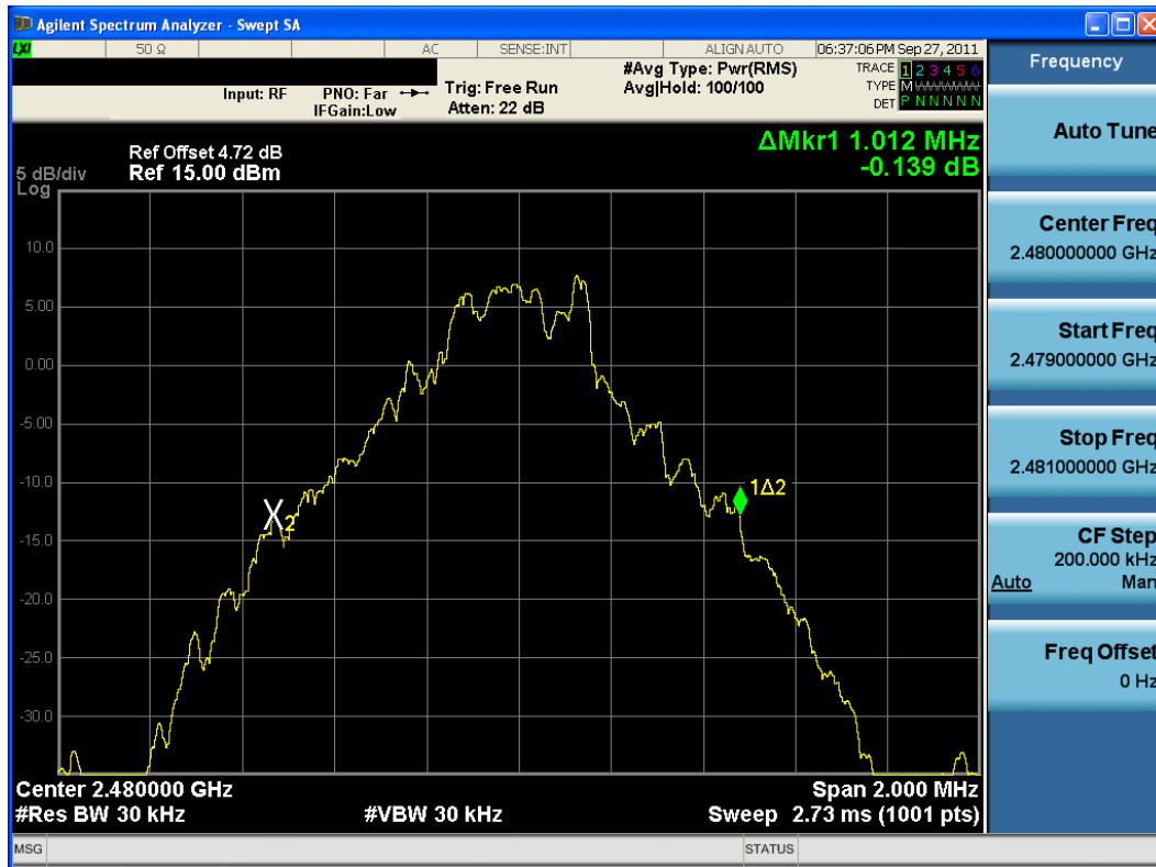
Plot 6-3. 20dB Bandwidth Plot (Bluetooth, 1Mbps – Ch. 78)
