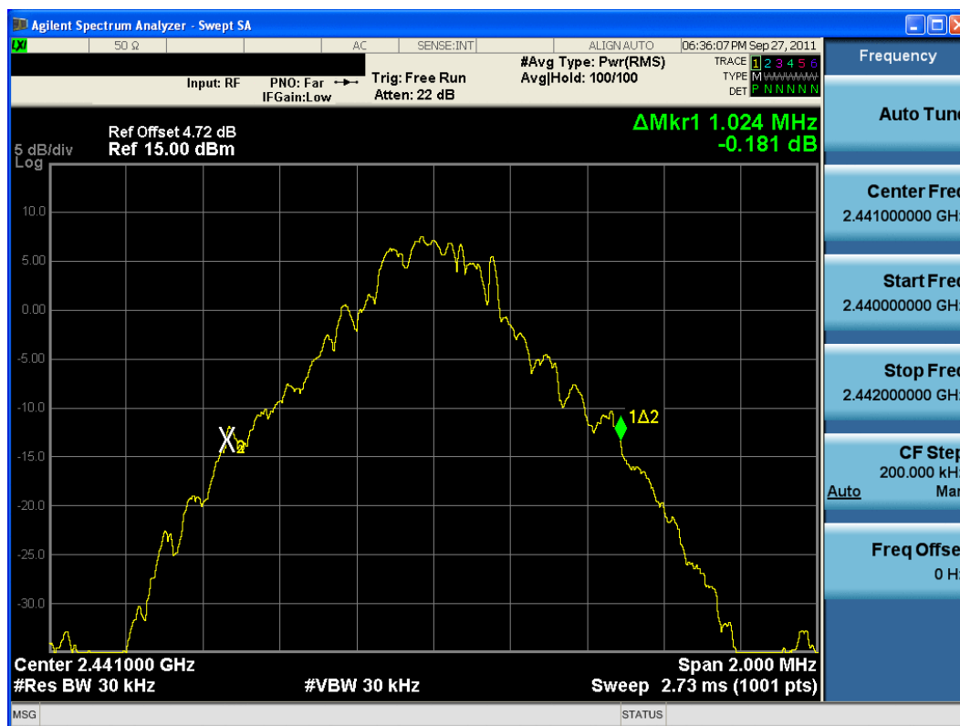
Plot 6-2. 20dB Bandwidth Plot (Bluetooth, 1Mbps – Ch. 39)
