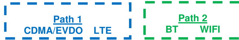
Figure 1-2 Simultaneous Transmission Paths
