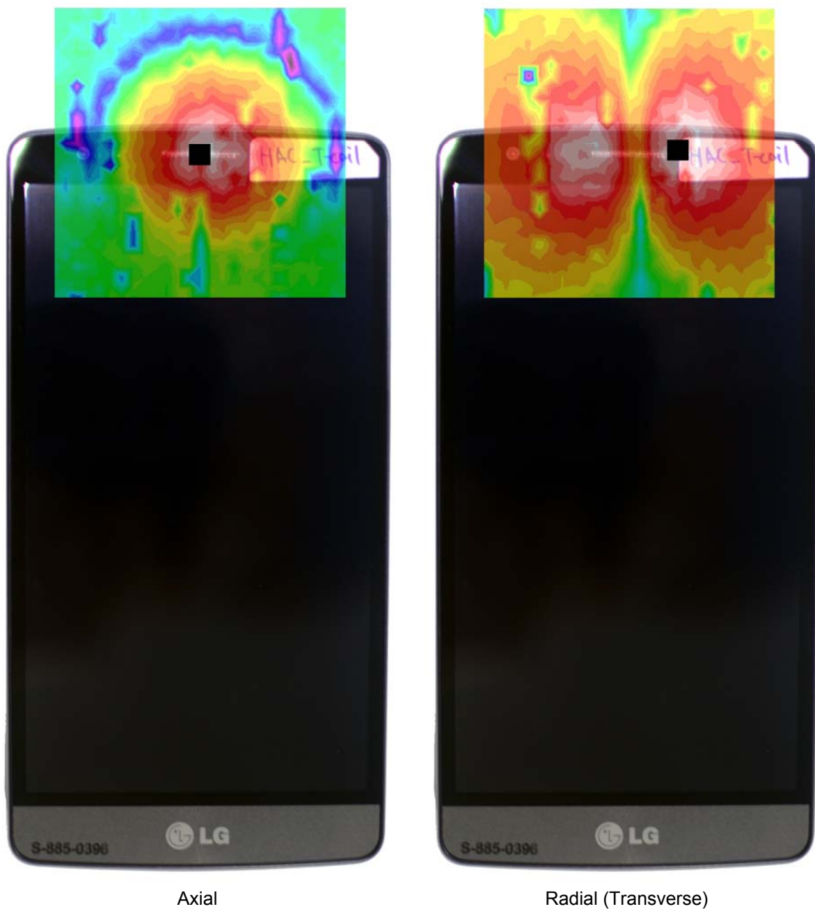
Figure 13-3 T-Coil Scan Overlay Magnetic Field Distributions
