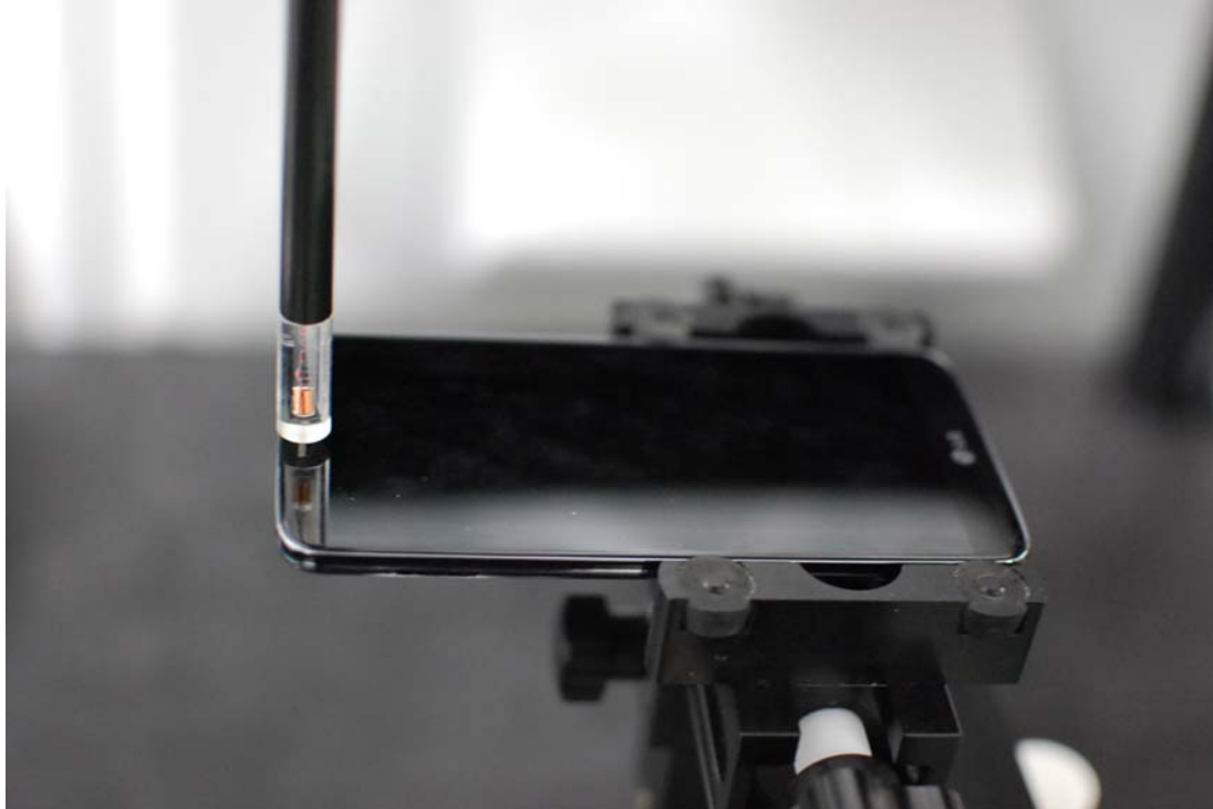
Figure 13-1 Test Setup for Wireless Device
