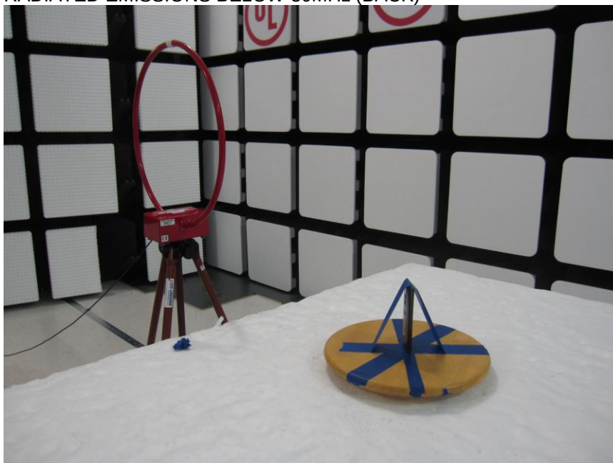
RADIATED EMISSIONS BELOW 30MHz (BACK)
