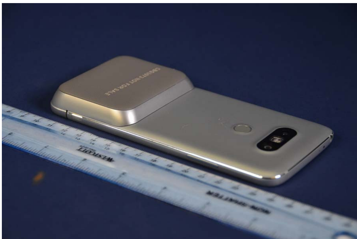
Camera Module Installed
