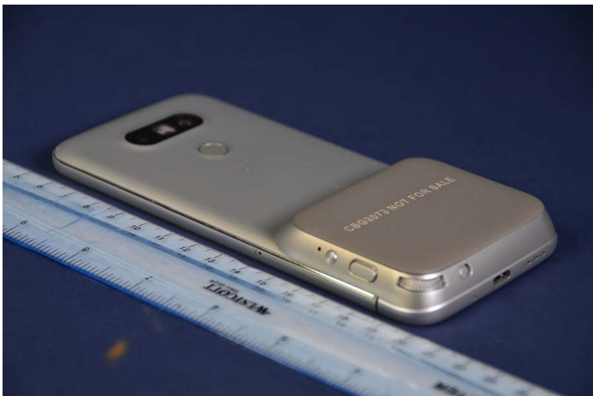
Camera Module Installed
