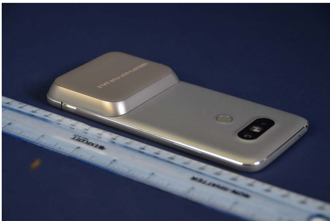
Camera Module Installed
