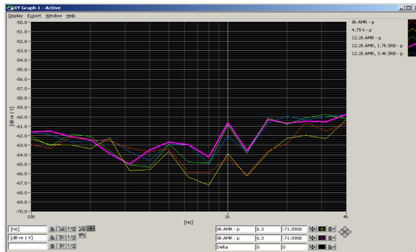
Figure 6-2 UMTS Audio Band Magnetic Noise
