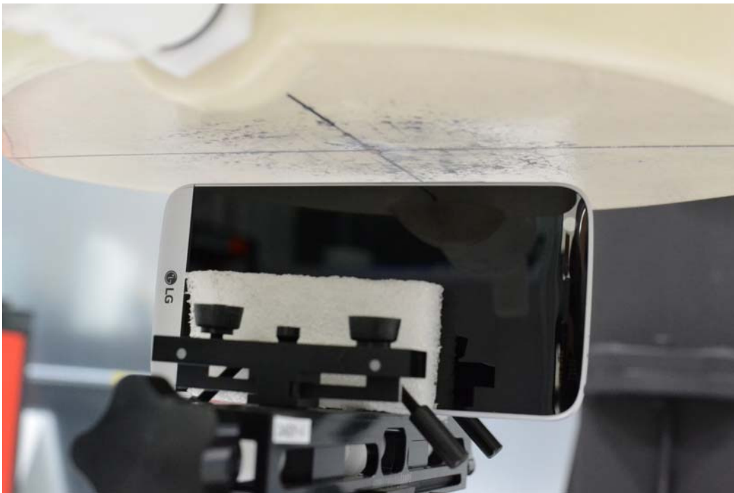
SAR Test Setup Photo 18: Left at 1.0 cm
