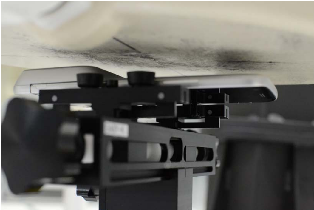
SAR Test Setup Photo 10: Back at 1.0 cm Camera Module Accessory
