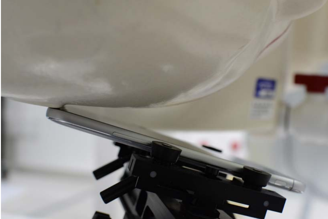
SAR Test Setup Photo 3: Right Tilt
