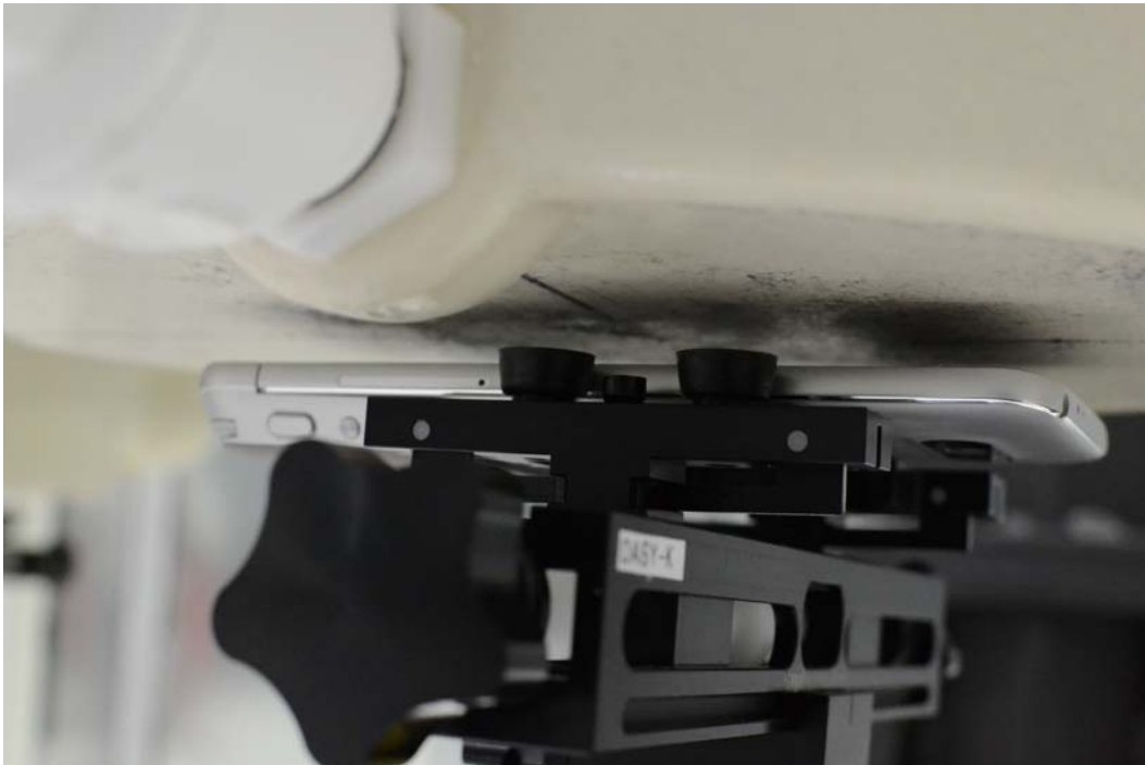
SAR Test Setup Photo 12: Front at 1.0 cm Camera Module Accessory
