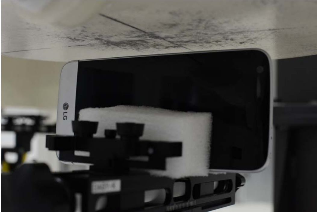
SAR Test Setup Photo 19: Left at 1.0 cm Camera Module Accessory
