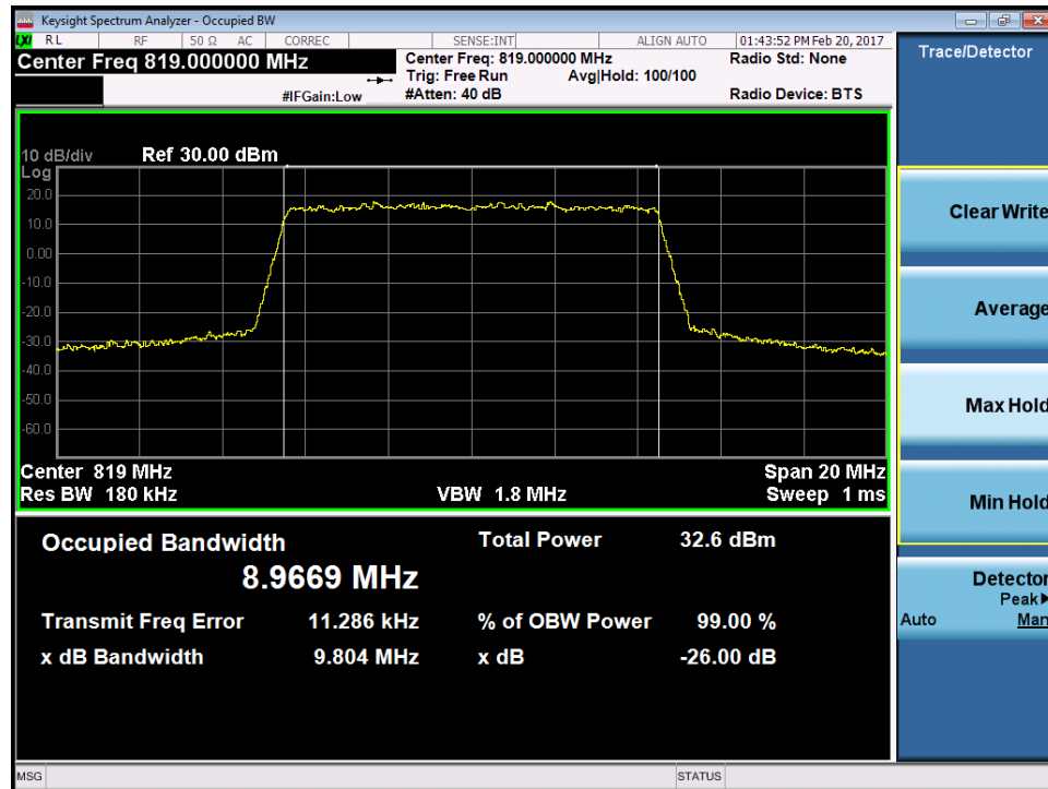
Plot 7-14. Occupied Bandwidth Plot LTE B26 (10MHz 64-QAM – RB Size 50)
