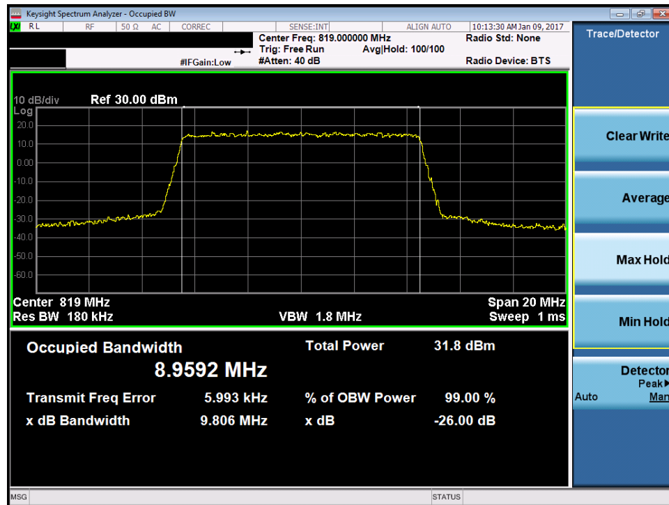
Plot 7-12. Occupied Bandwidth Plot LTE B26 (10MHz QPSK – RB Size 50)
