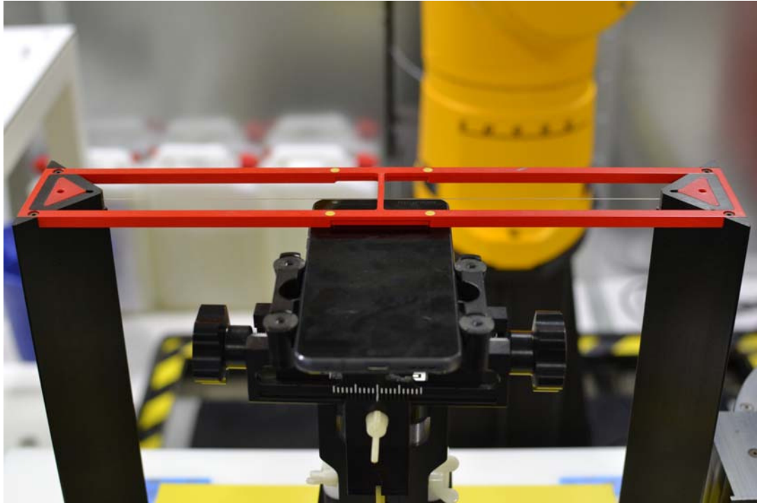
Figure 18-1 Ear Reference Point HAC Phantom Alignment
