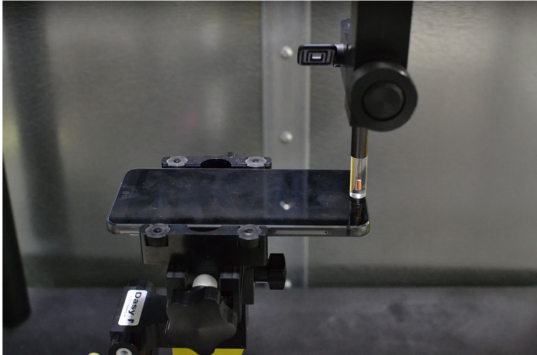
Figure 13-1 Test Setup for Wireless Device
