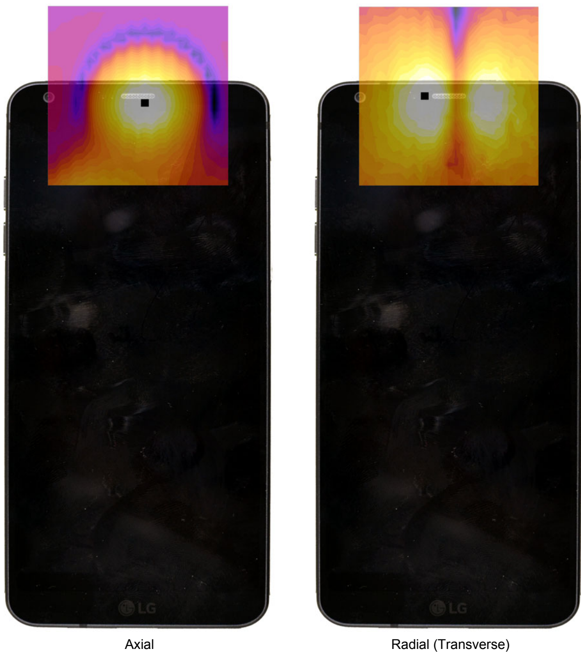
Figure 13-3 T-Coil Scan Overlay Magnetic Field Distributions
