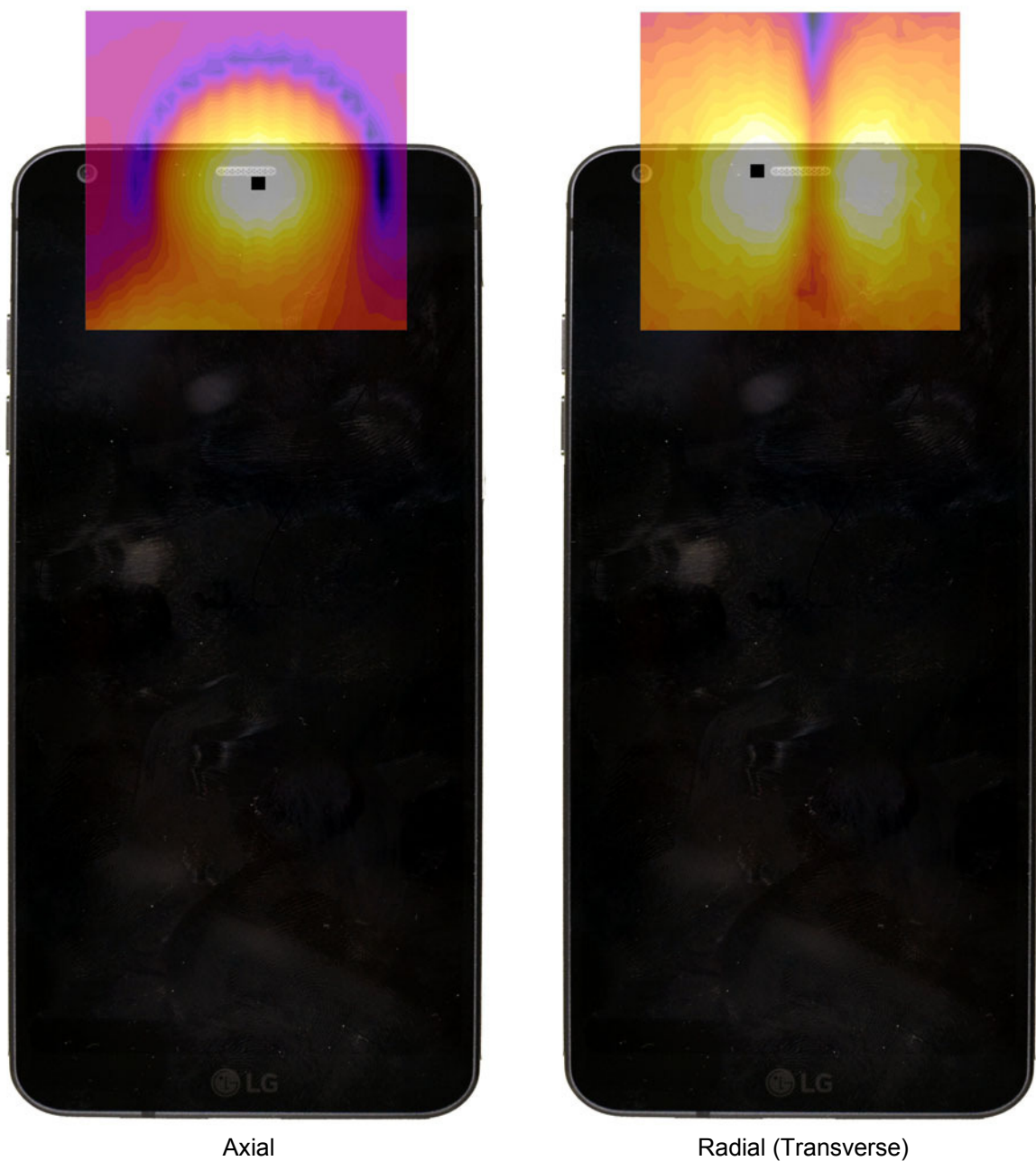
Figure 13-3 T-Coil Scan Overlay Magnetic Field Distributions
