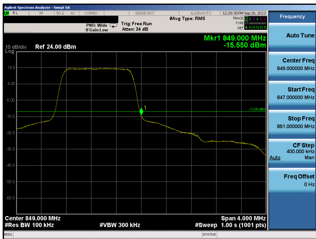
Plot 7-10. Upper Band Edge Plot (1.4MHz QPSK – RB Size 6)
