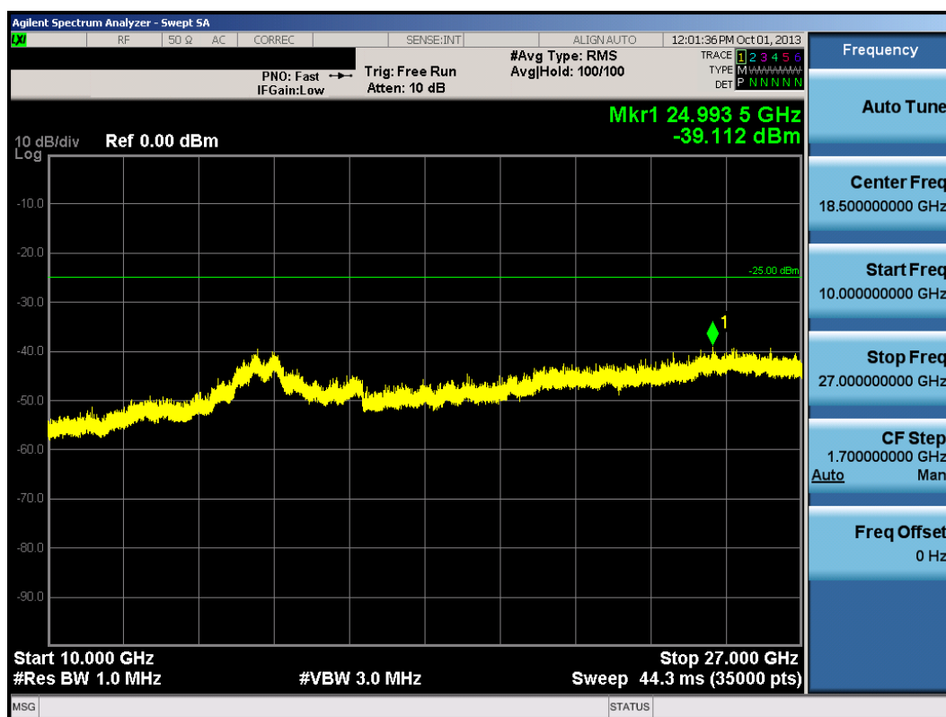
Plot 9-8. Conducted Spurious Plot (10.0MHz QPSK – RB Size 1, RB Offset 0 – Low Channel)
