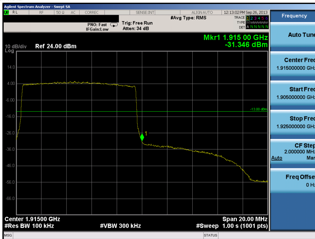
Plot 8-27. Upper Band Edge Plot (10.0MHz QPSK – RB Size 50)
