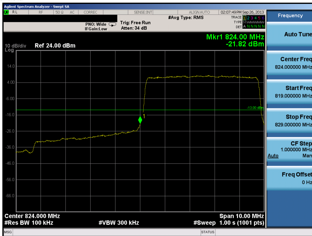
Plot 7-15. Lower Band Edge Plot (5.0MHz QPSK – RB Size 25)
