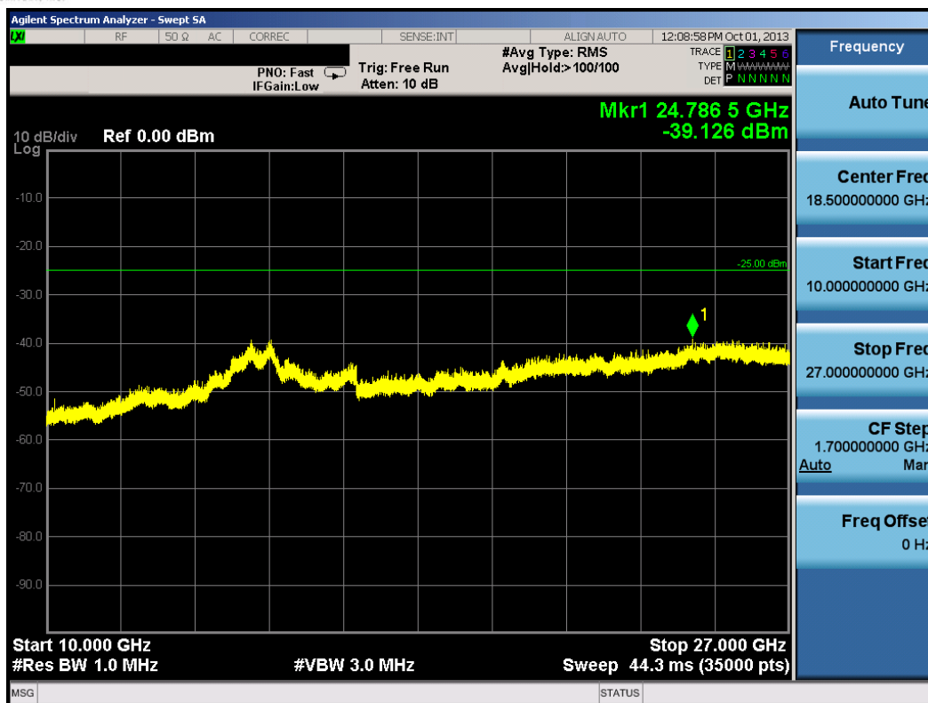
Plot 9-11. Conducted Spurious Plot (10.0MHz QPSK – RB Size 1, RB Offset 0 – Mid Channel)
