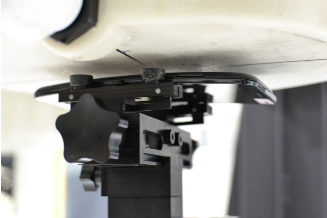
SAR Test Setup Photo 5 – Back Side at 0.8 cm
