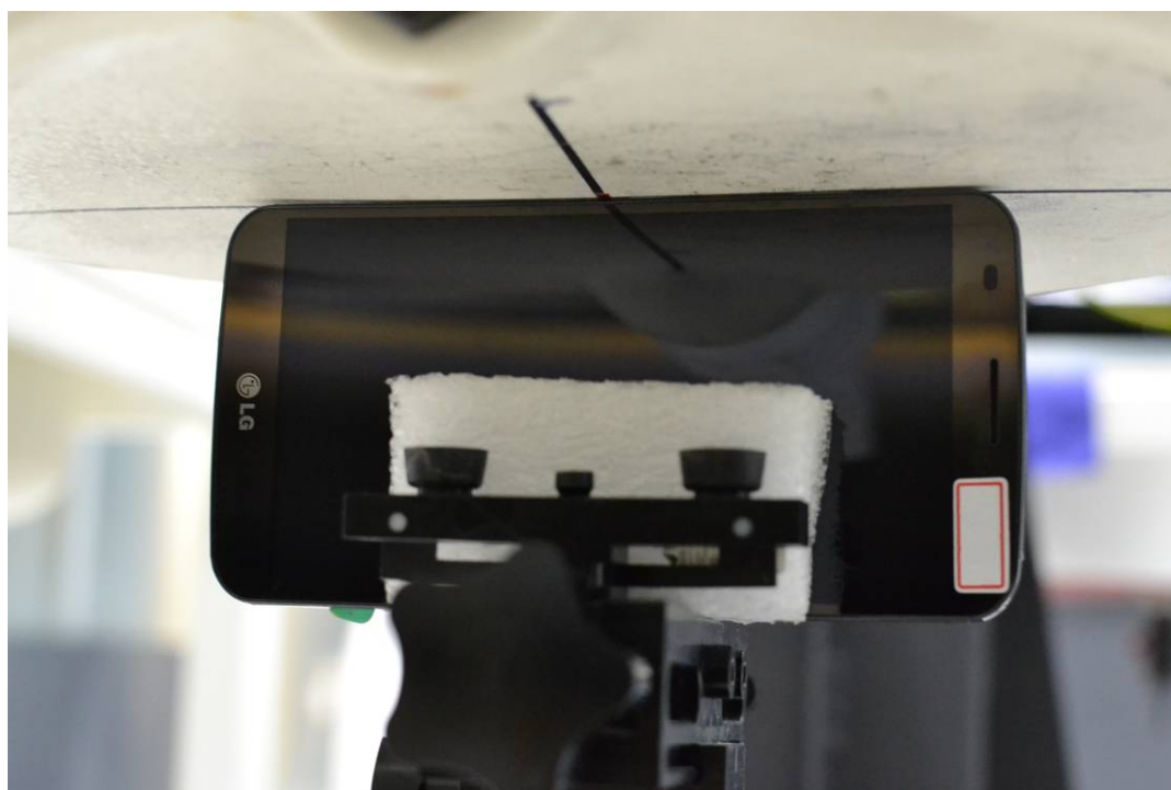
SAR Test Setup Photo 14 – Left Edge at 0.0 cm
