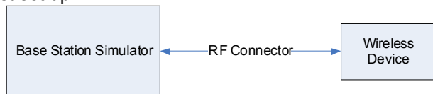
Figure 9-1 Power Measurement Setup
