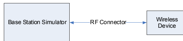
Figure 9-3 Power Measurement Setup
