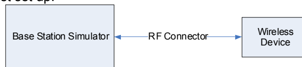
Figure 9-1 Power Measurement Setup
