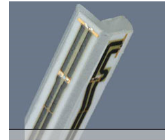
Figure 5-1 E-field Free-space Probe
