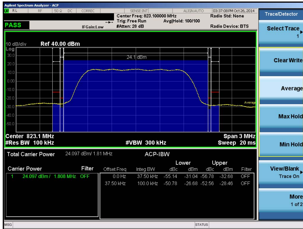
Plot 7-6. Channel Edge Plot (Ch. 684)
