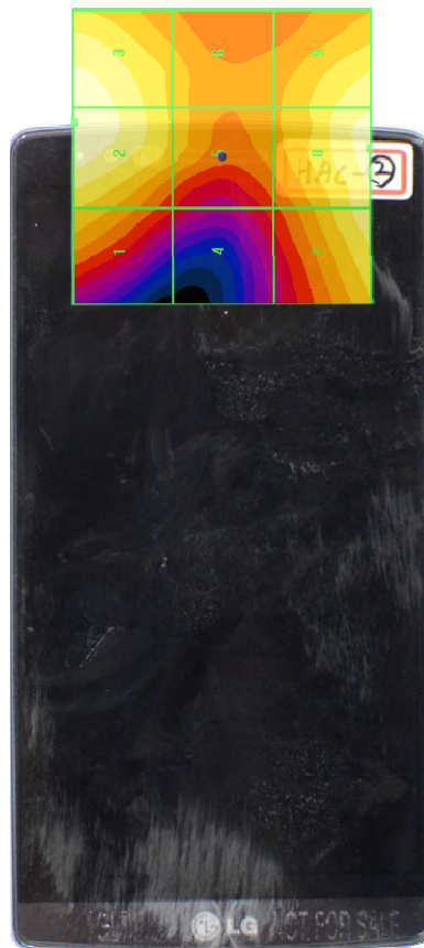
Figure 18-4 E-Field WD Scan overlay
