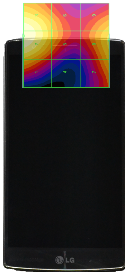
Figure 18-4 E-Field WD Scan overlay
