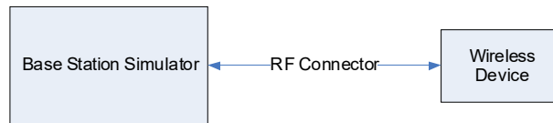
Figure 9-3 Power Measurement Setup
