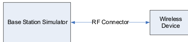
Figure 9-4 Power Measurement Setup
