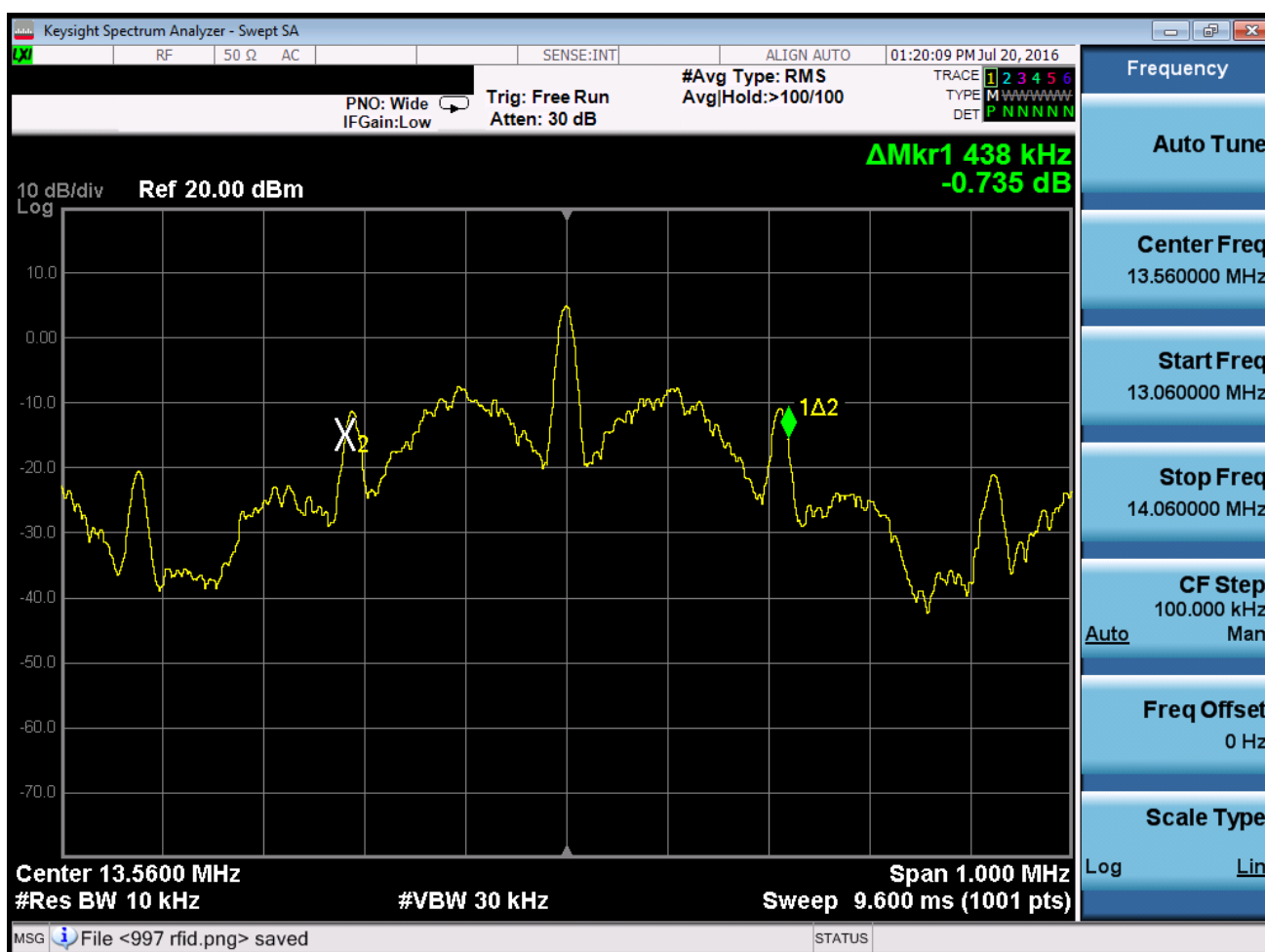
Figure 8-2. 20dB Bandwidth Plot
