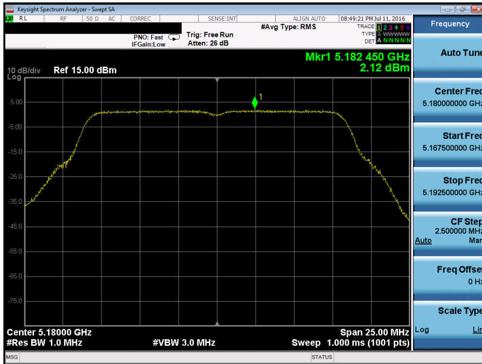
Plot 7-115. Power Spectral Density Plot (802.11a (UNII Band 1) – Ch. 36)
