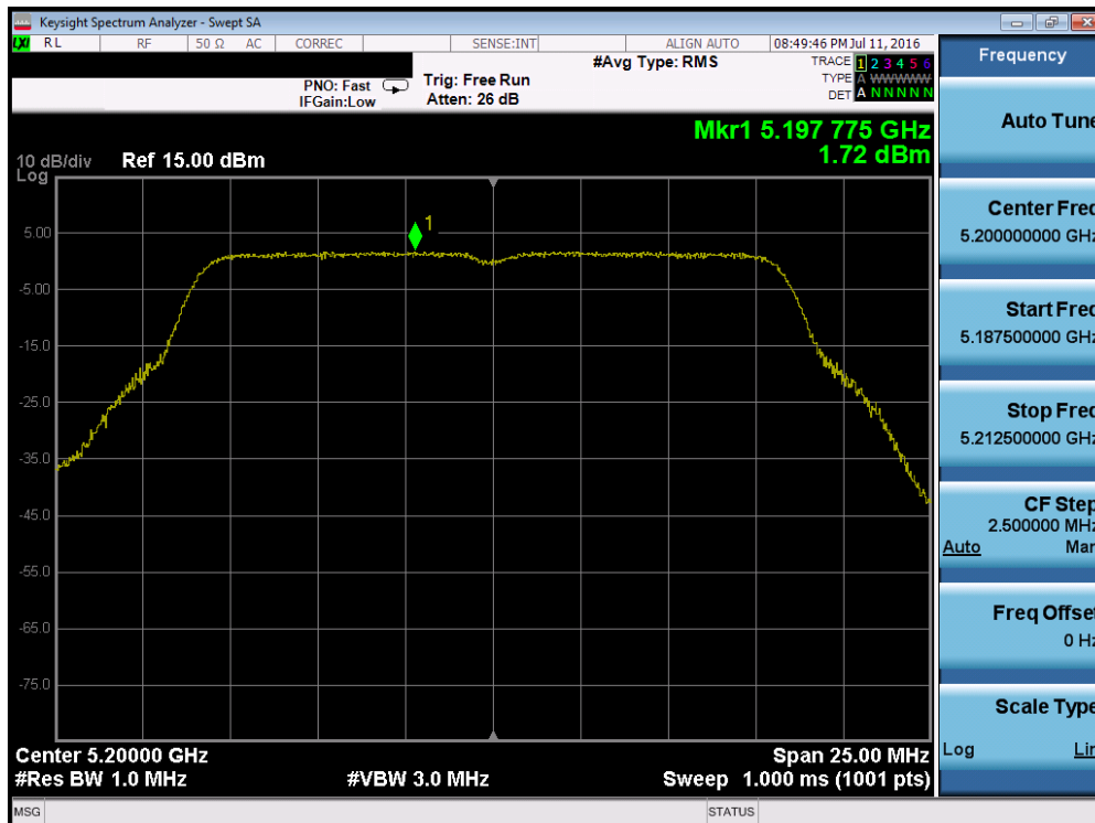
Plot 7-116. Power Spectral Density Plot (802.11a (UNII Band 1) – Ch. 40)
