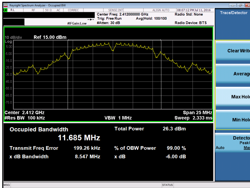
Plot 7-10. 6dB Bandwidth Plot (802.11b – Ch. 1)
