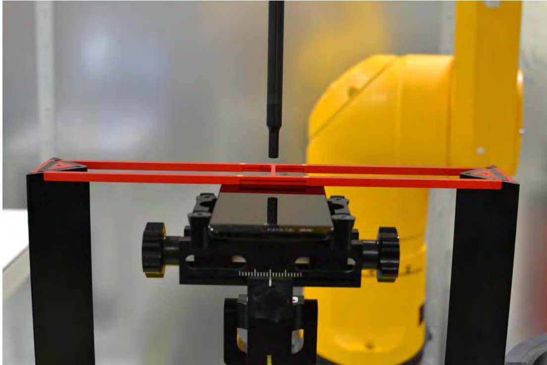
Figure 17-1 Ear Reference Point HAC Phantom Alignment
