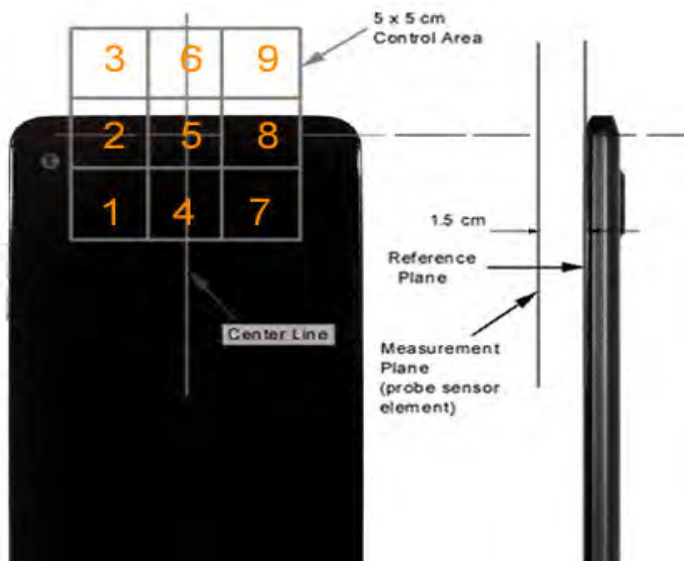
Figure 17-3 5x5 Scan grid above WD
