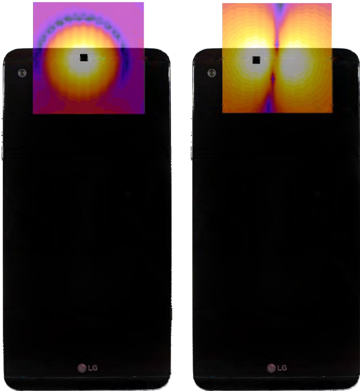
Figure 13-3 T-Coil Scan Overlay Magnetic Field Distributions
