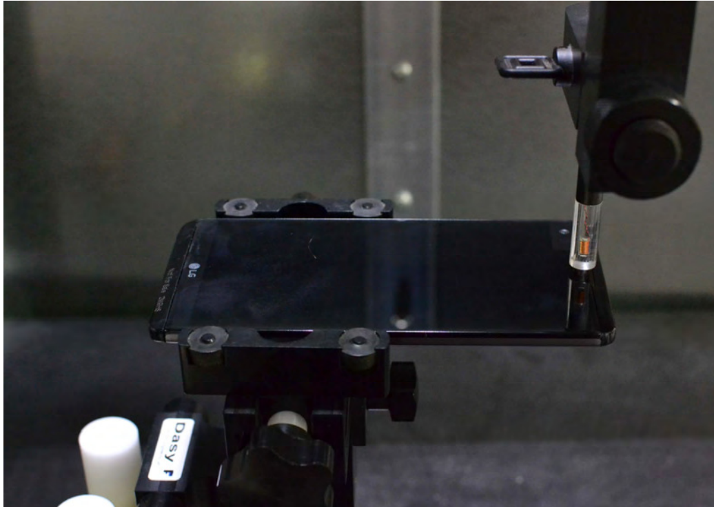
Figure 13-1 Test Setup for Wireless Device
