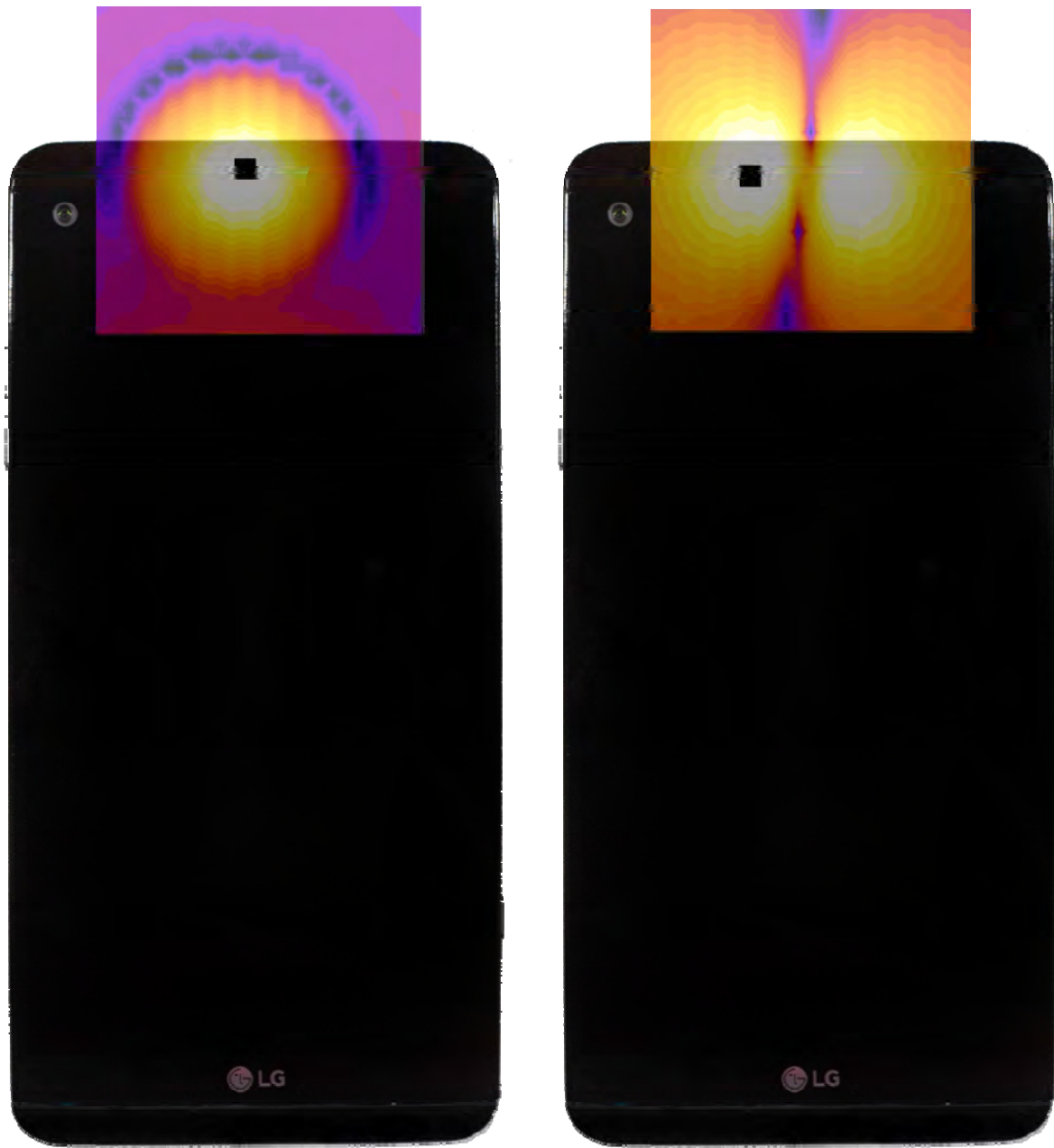
Figure 13-3 T-Coil Scan Overlay Magnetic Field Distributions
