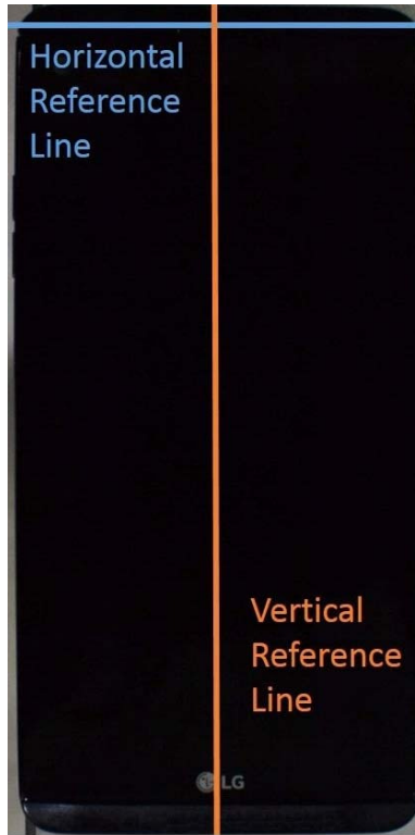
SAR Test Setup Photo 15: Horizontal and Vertical Reference Lines
