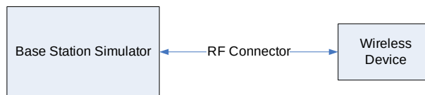
Figure 9-2 Power Measurement Setup
