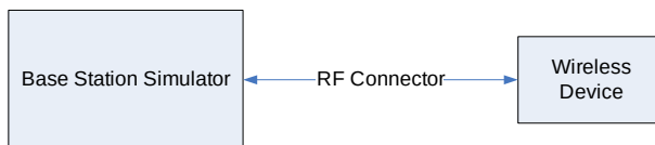
Figure 9-1 Power Measurement Setup
