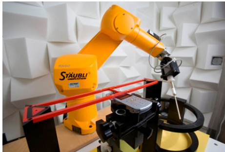
Figure 4-3 SPEAG Robotic System
