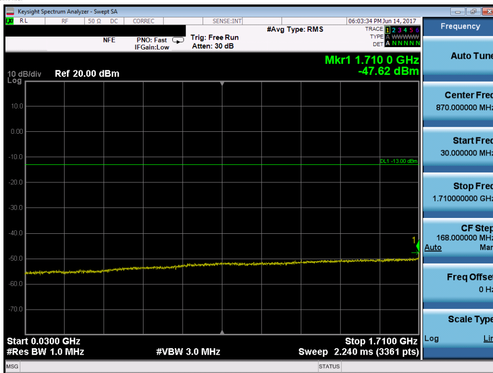
Plot 7-106. Conducted Spurious Plot (Band 4 – 10.0MHz QPSK – RB Size 1, RB Offset 0 – Mid Channel)
