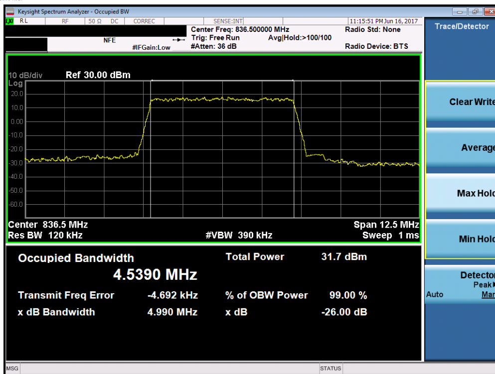
Plot 7-25. Occupied Bandwidth Plot (Band 5/26 – 5.0MHz QPSK – RB Size 25)
