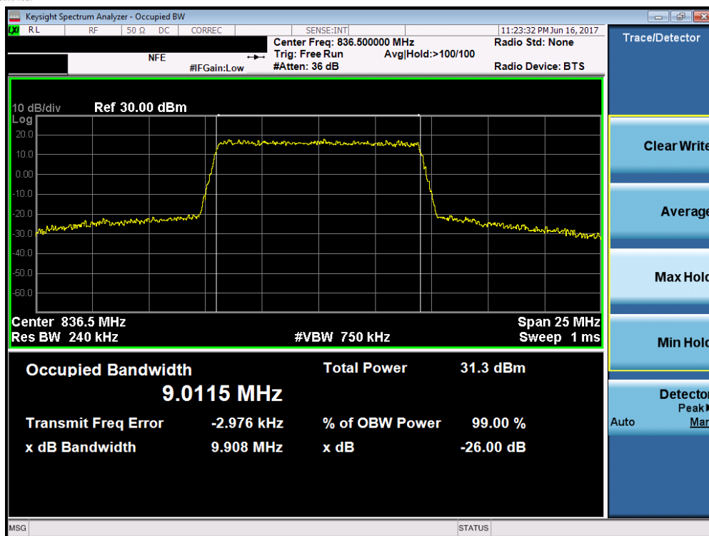
Plot 7-29. Occupied Bandwidth Plot (Band 5/26 – 10.0MHz 16-QAM – RB Size 50)
