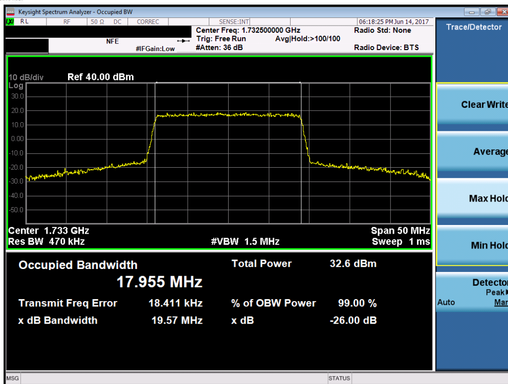
Plot 7-49. Occupied Bandwidth Plot (Band 4 – 20.0MHz QPSK – RB Size 100)
