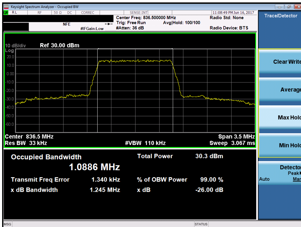
Plot 7-20. Occupied Bandwidth Plot (Band 5/26 – 1.4MHz 16-QAM – RB Size 6)
