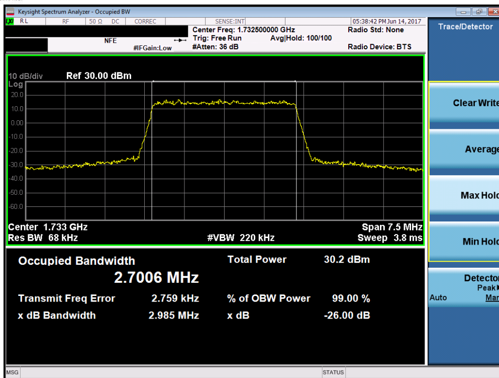
Plot 7-39. Occupied Bandwidth Plot (Band 4 – 3.0MHz 64-QAM – RB Size 15)
