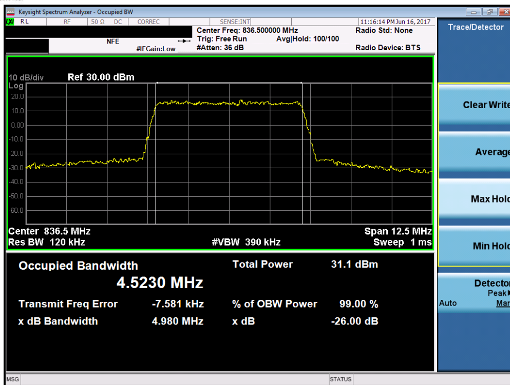
Plot 7-27. Occupied Bandwidth Plot (Band 5/26 – 5.0MHz 64-QAM – RB Size 25)
