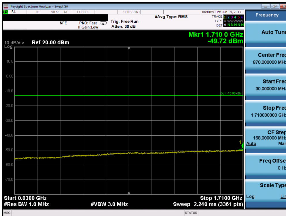
Plot 7-109. Conducted Spurious Plot (Band 4 – 10.0MHz QPSK – RB Size 1, RB Offset 0 – High Channel)
