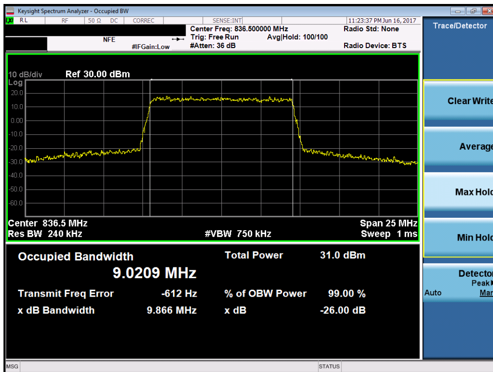
Plot 7-30. Occupied Bandwidth Plot (Band 5/26 – 10.0MHz 64-QAM – RB Size 50)
