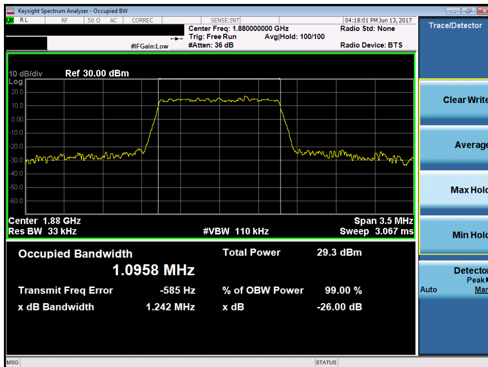
Plot 7-54. Occupied Bandwidth Plot (Band 2/25 – 1.4MHz 64-QAM – RB Size 6)
