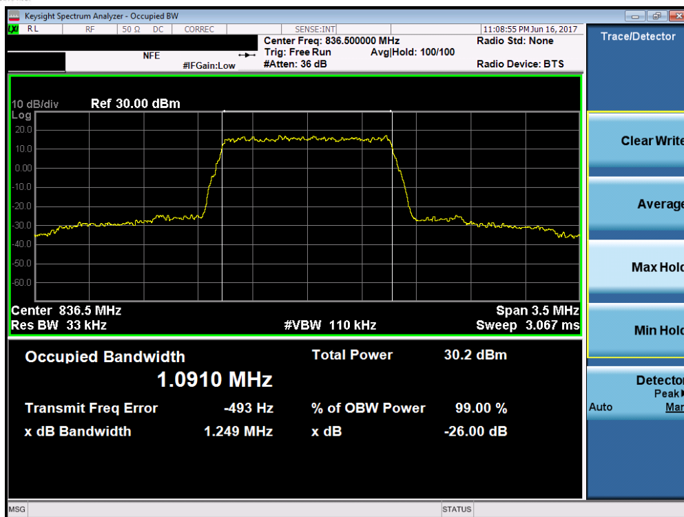
Plot 7-21. Occupied Bandwidth Plot (Band 5/26 – 1.4MHz 64-QAM – RB Size 6)
