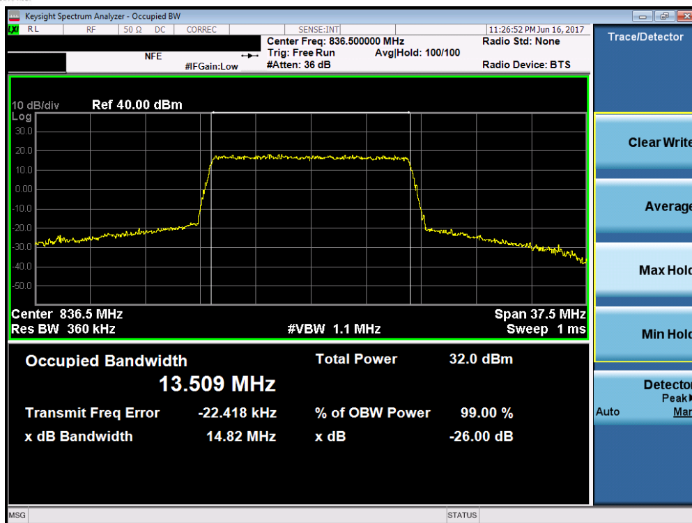
Plot 7-31. Occupied Bandwidth Plot (Band 5/26 - 15.0MHz QPSK - RB Size 75)
