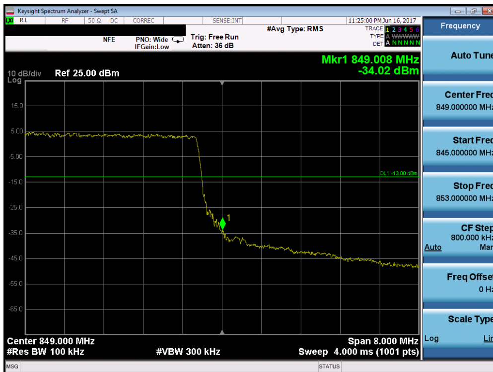
Plot 7-155. Upper Band Edge Plot (Band 5/26 - 10.0MHz QPSK - RB Size 50)
