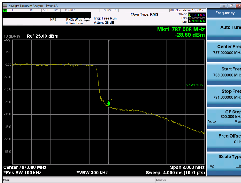
Plot 7-146. Upper Band Edge Plot (Band 13 – 10.0MHz QPSK – RB Size 50)
