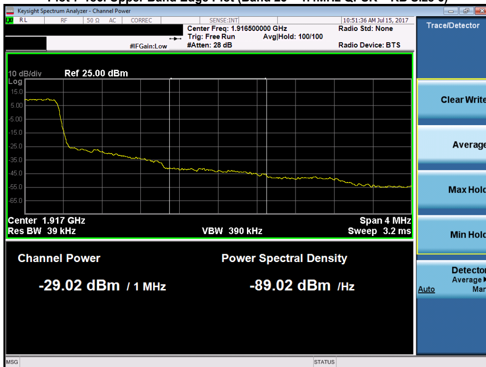
Plot 7-187. Upper Extended Band Edge Plot (Band 25 – 1.4MHz QPSK – RB Size 6)
