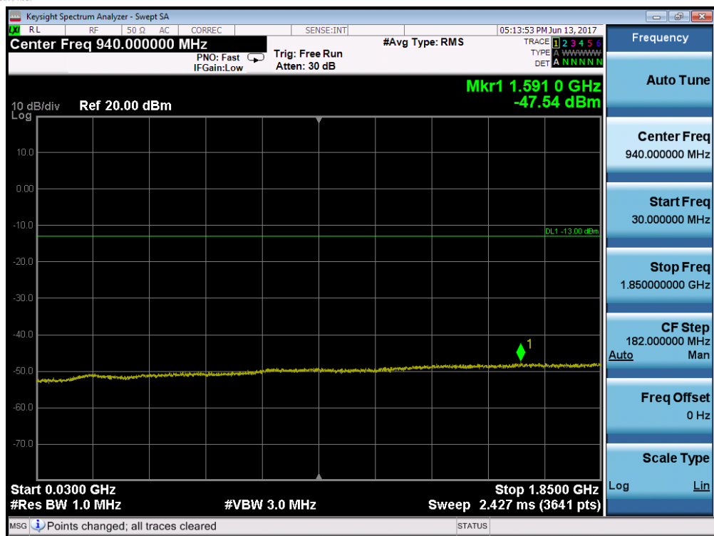
Plot 7-118. Conducted Spurious Plot (Band 2/25 – 5.0MHz QPSK – RB Size 1, RB Offset 0 – High Channel)
