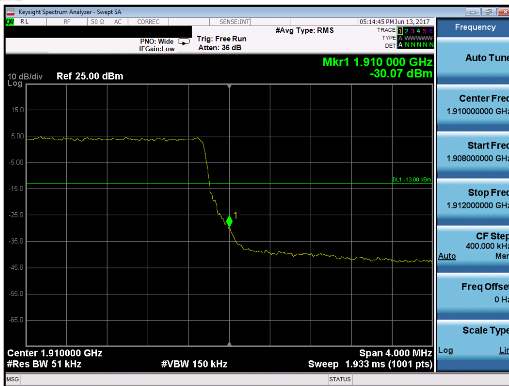
Plot 7-196. Upper Band Edge Plot (Band 2 – 5.0MHz QPSK – RB Size 25)
