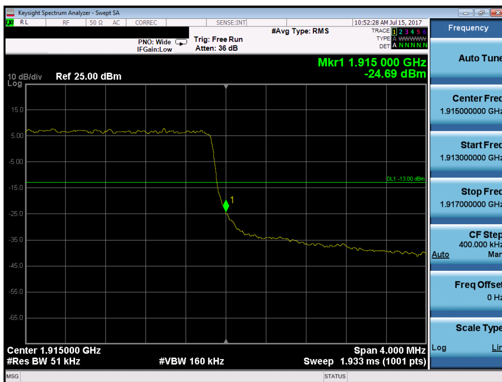
Plot 7-192. Upper Band Edge Plot (Band 25 – 3.0MHz QPSK – RB Size 15)
