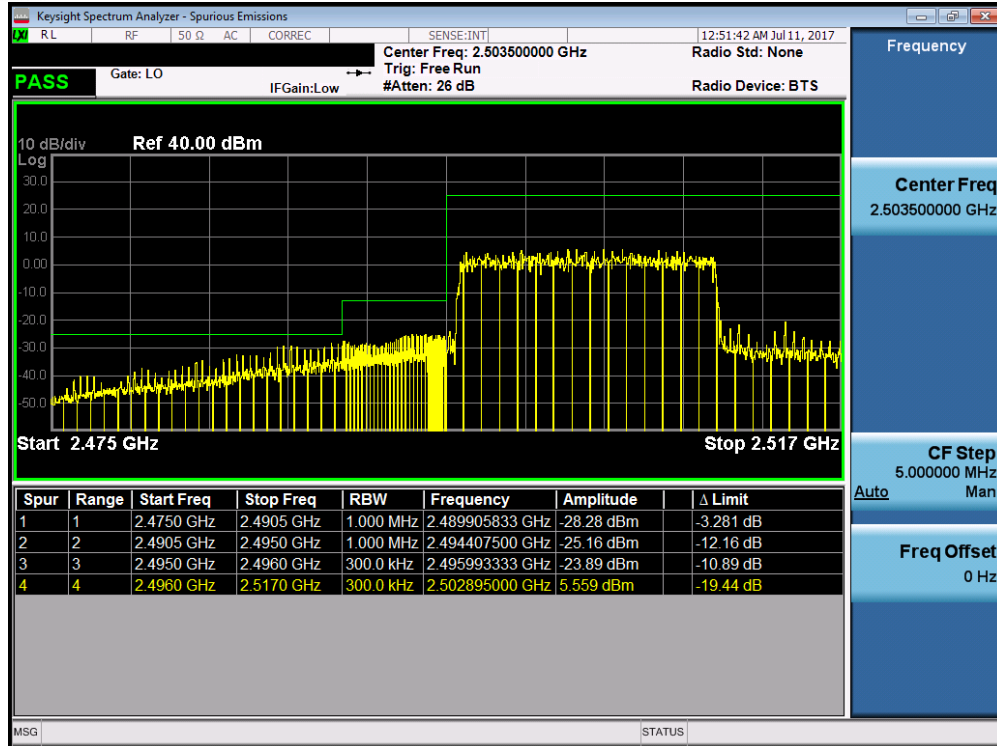
Plot 7-222. Lower ACP Plot (Band 41 – 15.0MHz QPSK – RB Size 75)
