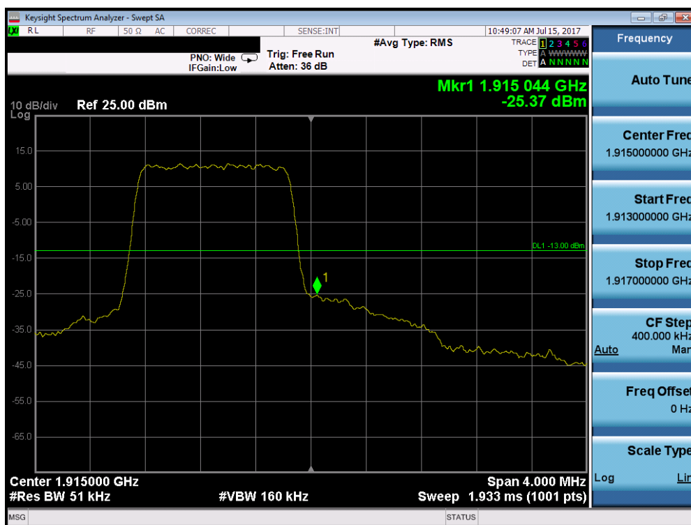
Plot 7-186. Upper Band Edge Plot (Band 25 – 1.4MHz QPSK – RB Size 6)
