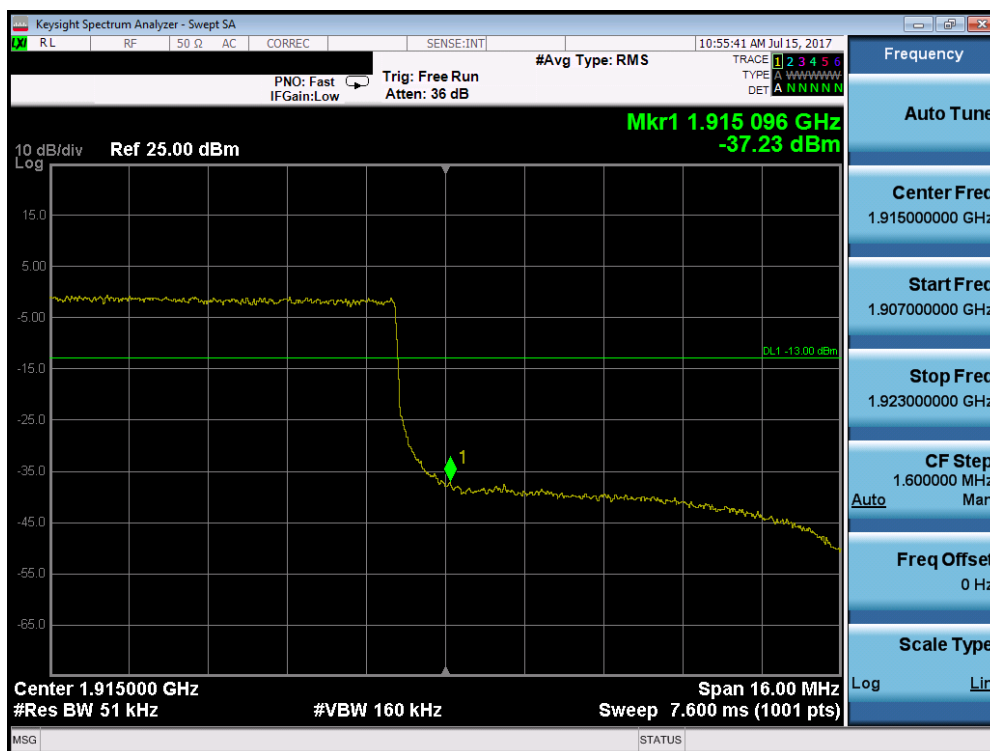
Plot 7-216. Upper Band Edge Plot (Band 25 – 20.0MHz QPSK – RB Size 100)
