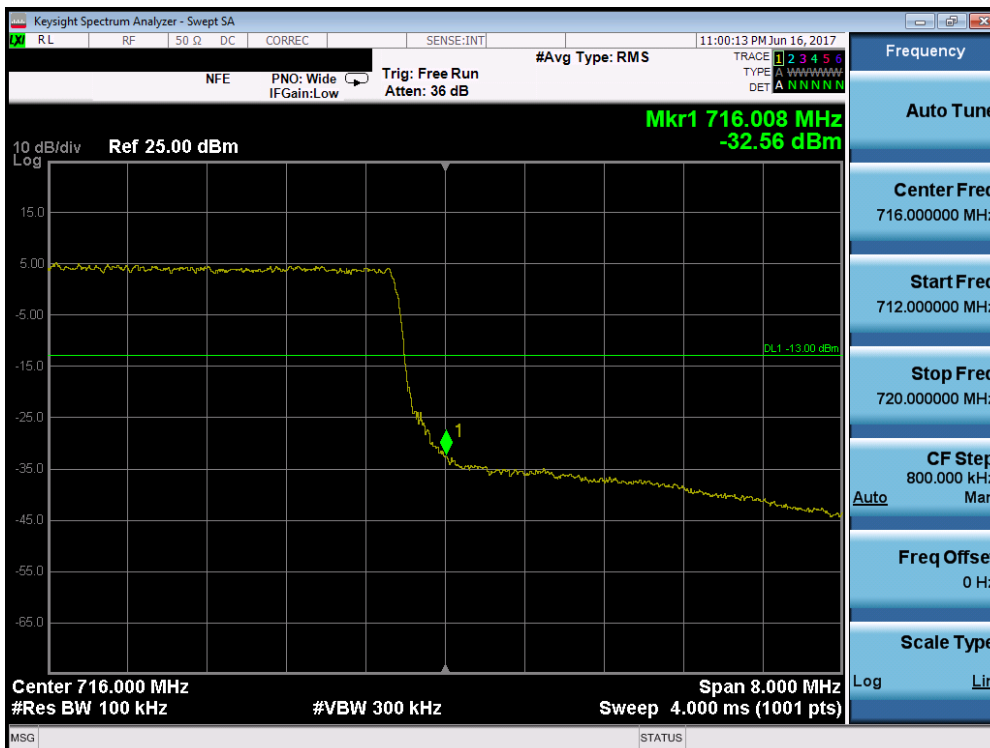
Plot 7-139. Upper Band Edge Plot (Band 12/17 – 10.0MHz QPSK – RB Size 50)
