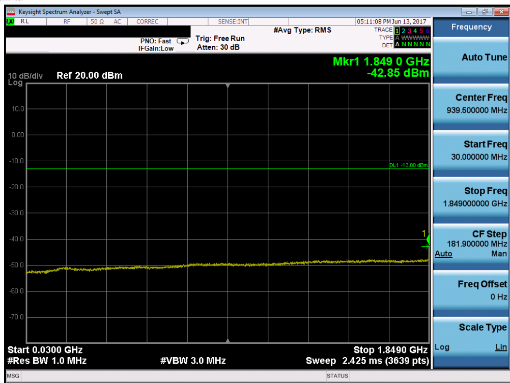
Plot 7-112. Conducted Spurious Plot (Band 2/25 – 5.0MHz QPSK – RB Size 1, RB Offset 0 – Low Channel)
