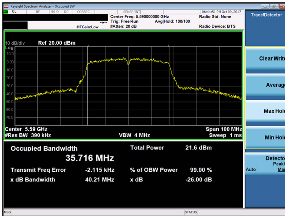
Plot 7-3. 26dB Bandwidth Plot (40MHz BW 802.11n (UNII Band 2C) – Ch. 118)
