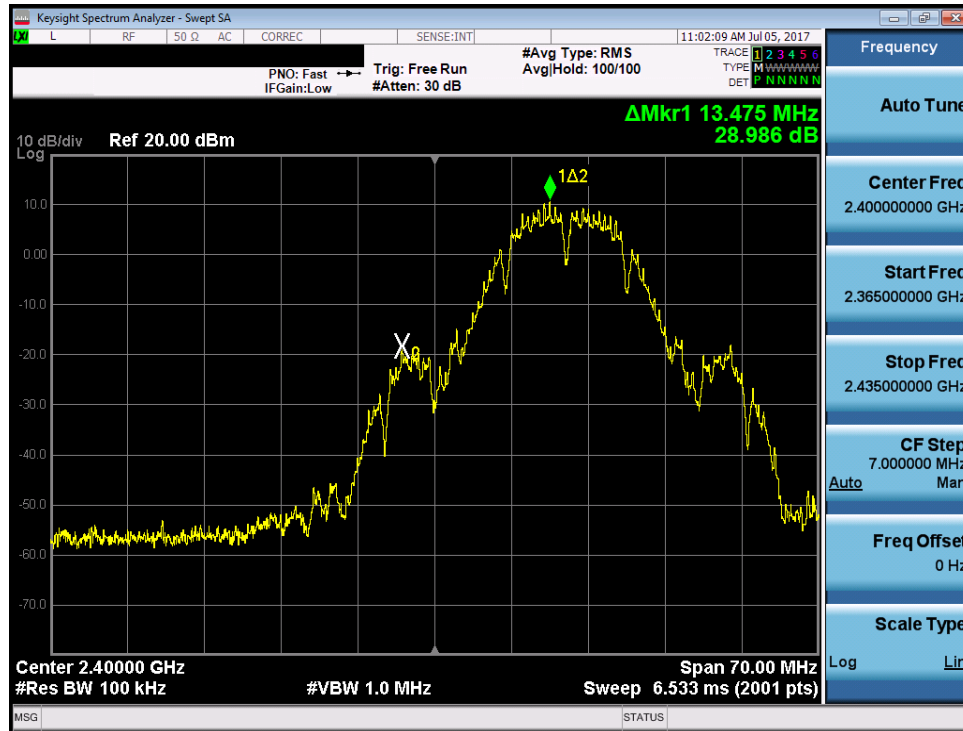
Plot 7-43. Band Edge Plot (802.11b – Ch. 1)
