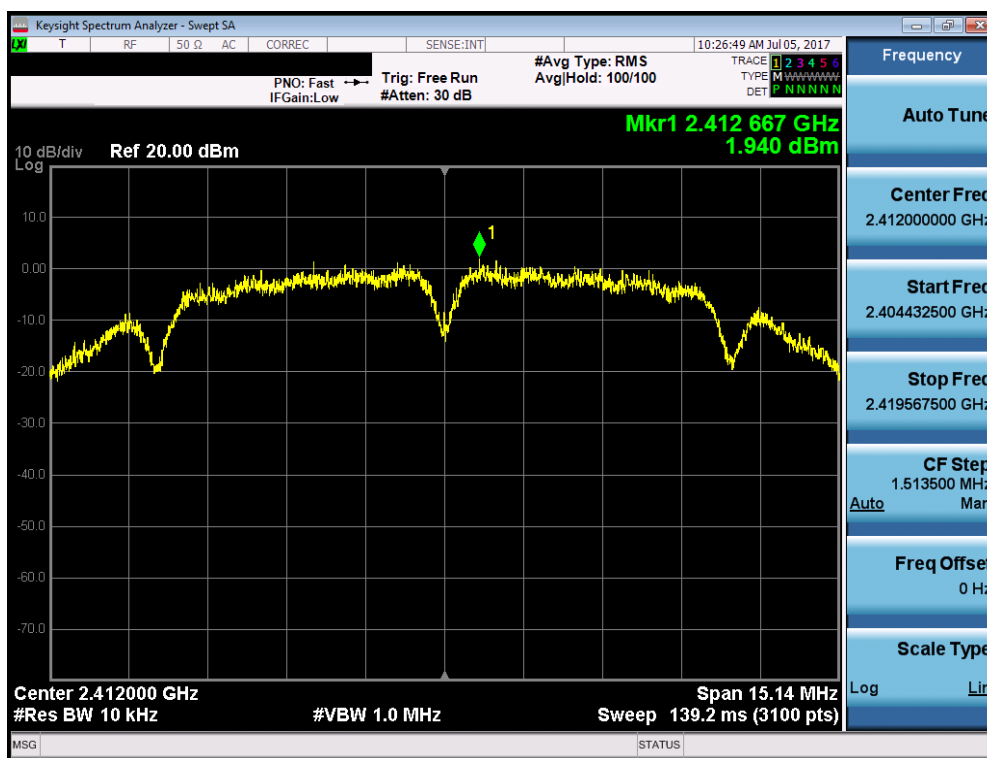
Plot 7-19. Power Spectral Density Plot (802.11b – Ch. 1)
