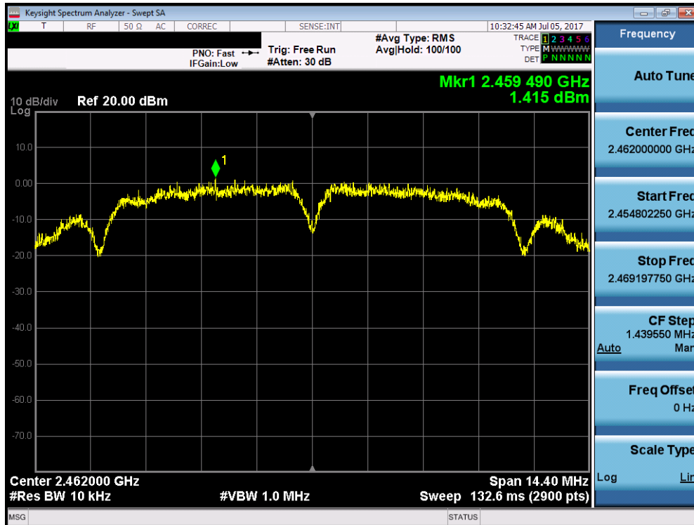
Plot 7-21. Power Spectral Density Plot (802.11b – Ch. 11)
