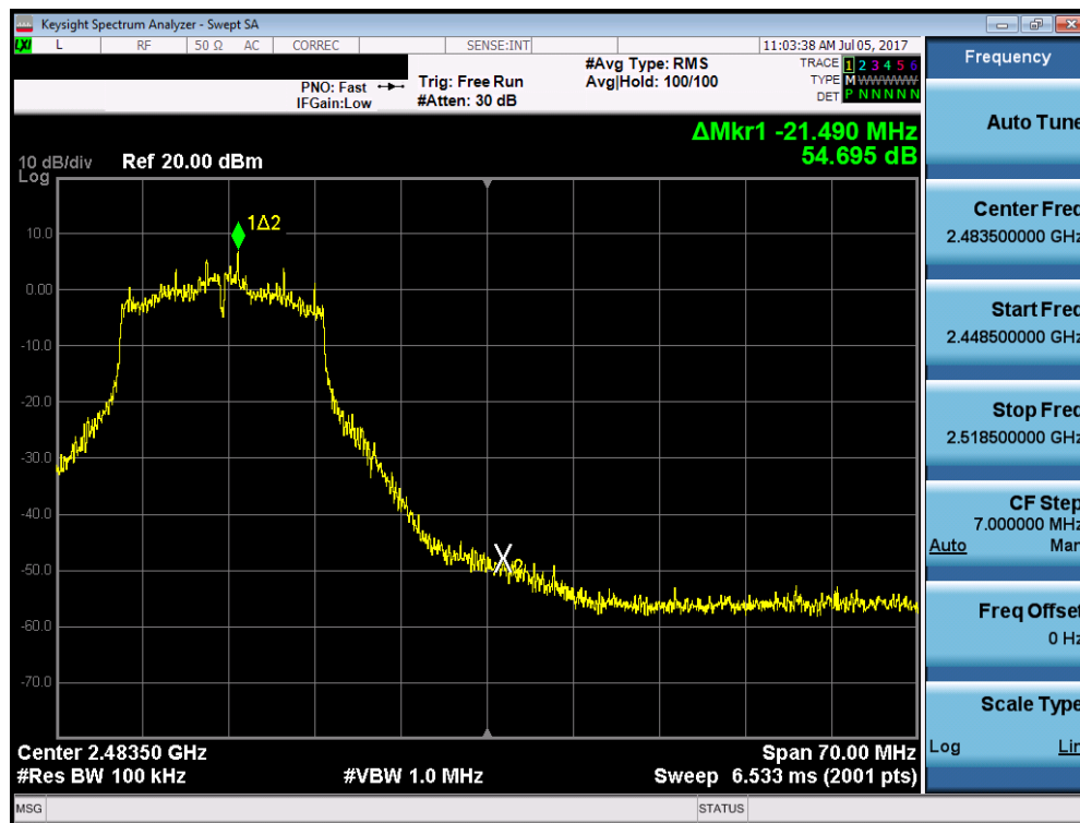
Plot 7-46. Band Edge Plot (802.11g - Ch. 11)
