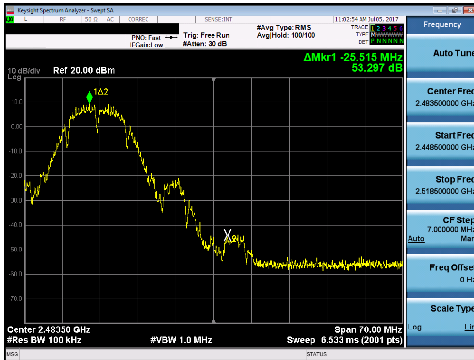
Plot 7-44. Band Edge Plot (802.11b – Ch. 11)
