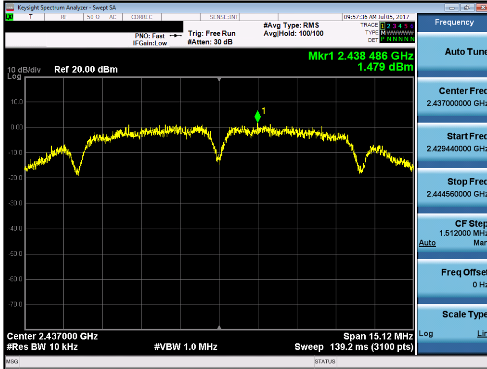
Plot 7-29. Power Spectral Density Plot (802.11b – Ch. 6)
