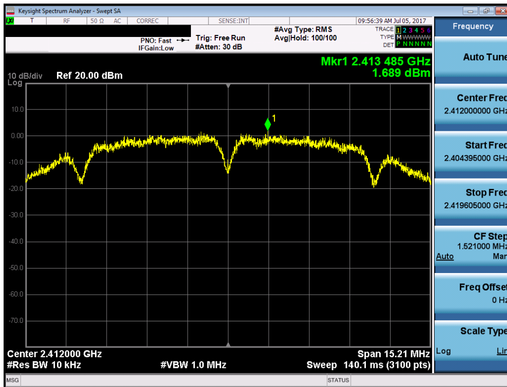
Plot 7-28. Power Spectral Density Plot (802.11b – Ch. 1)
