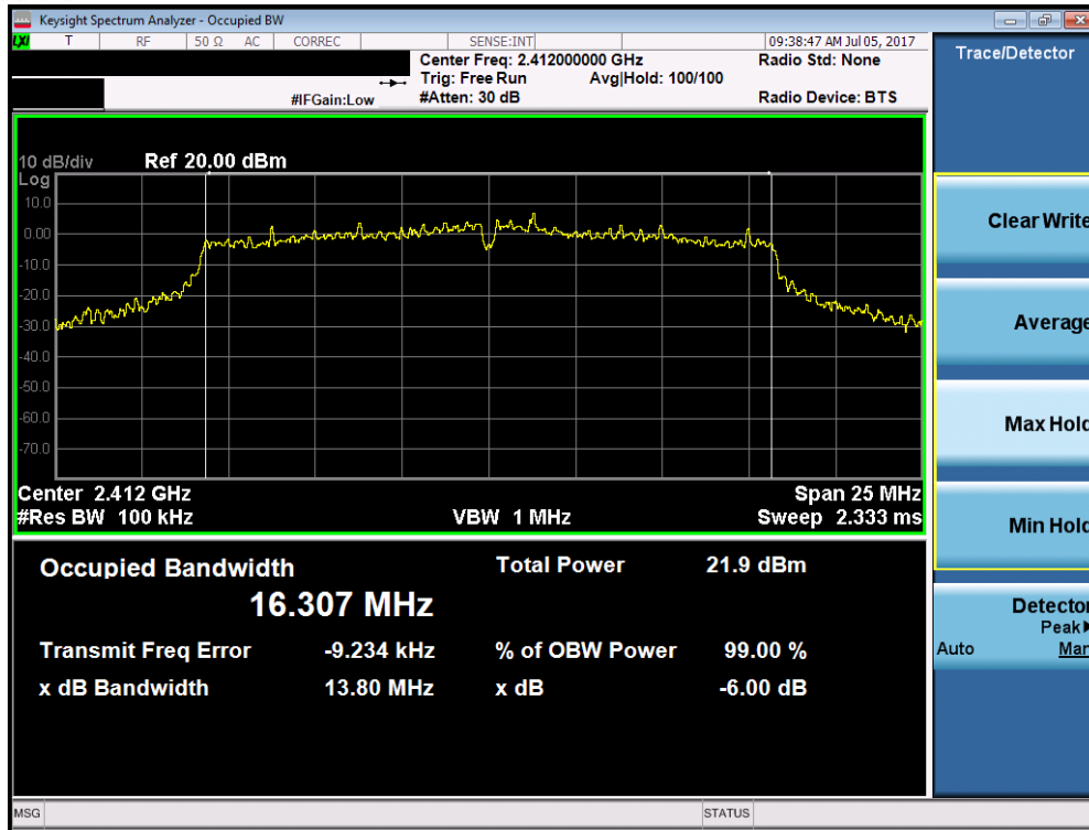
Plot 7-13. 6dB Bandwidth Plot (802.11g – Ch. 1)
