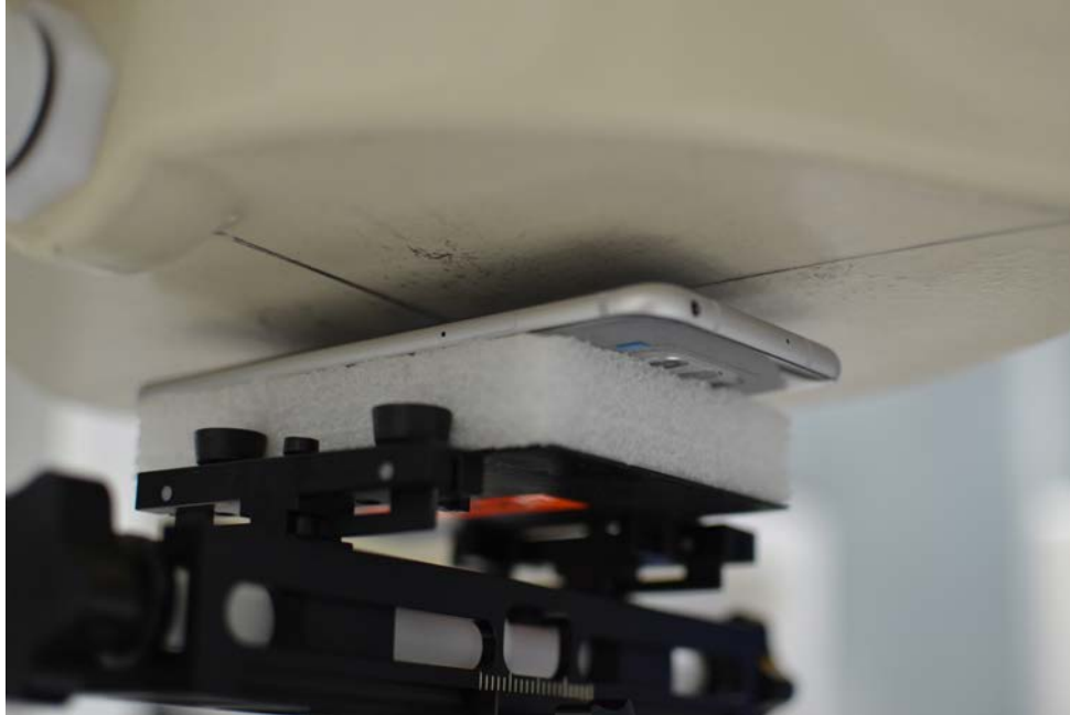
SAR Test Setup Photo 7: Front at 1.0 cm
