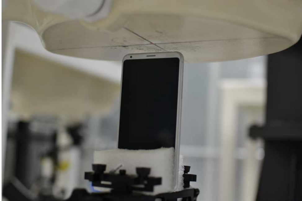
SAR Test Setup Photo 9: Top at 1.0 cm
