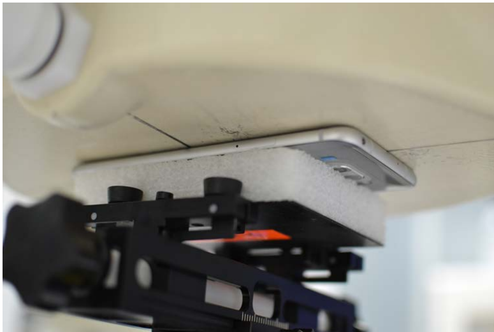
SAR Test Setup Photo 8: Front at 0.0 cm
