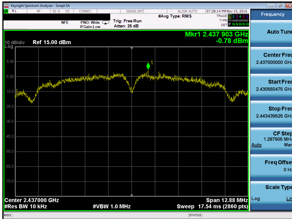
Plot 7-11. Power Spectral Density Plot (802.11b – Ch. 6)
