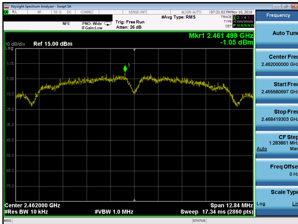
Plot 7-12. Power Spectral Density Plot (802.11b – Ch. 11)
