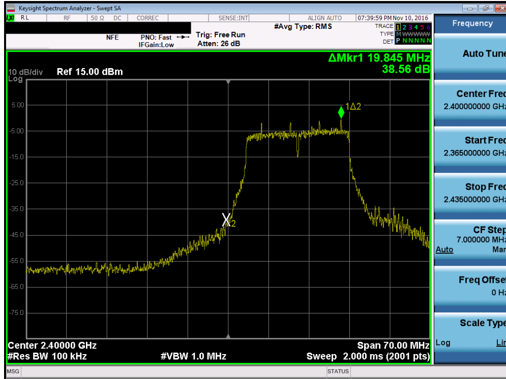
Plot 7-23. Band Edge Plot (802.11n (2.4GHz) – Ch. 1)
