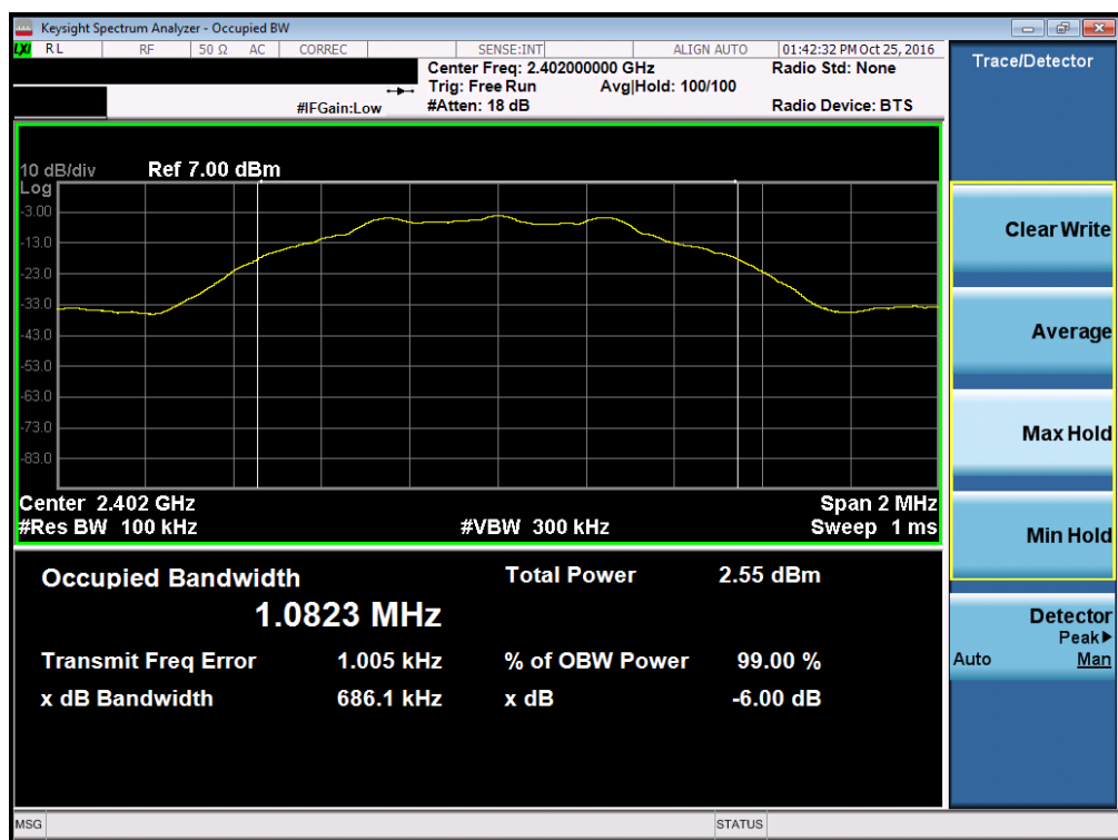
Plot 7-1. 6dB Bandwidth Plot (Bluetooth (LE) – Ch. 0)
