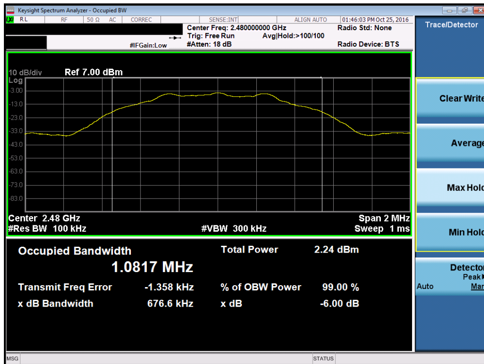
Plot 7-3. 6dB Bandwidth Plot (Bluetooth (LE) – Ch. 39)
