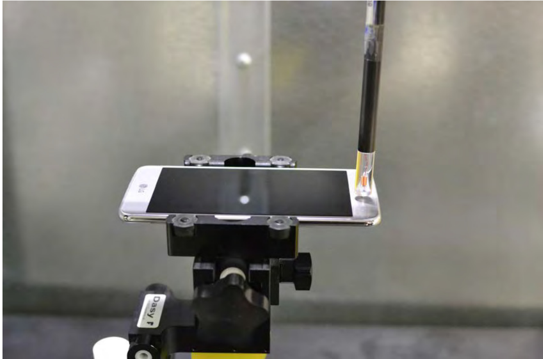
Figure 13-1 Test Setup for Wireless Device
